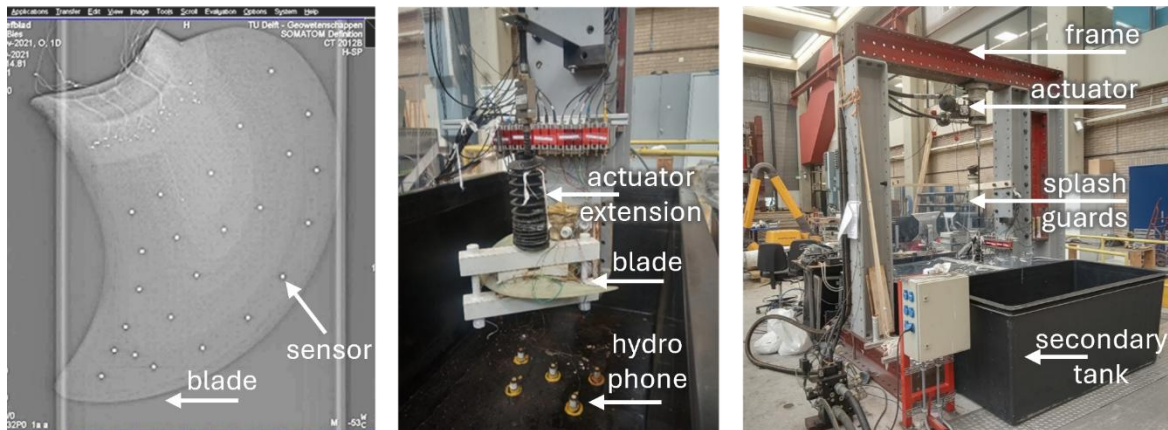
Fig. 2 Assessment of a composite marine propeller blade. The left picture visualises CT-scanning of the blade. In the middle a photograph is shown of the blade in the fatigue set-up, including the hydrophones mounted underneath the blade. The right picture shows the full experimental setup with secondary tank and splash guards.
