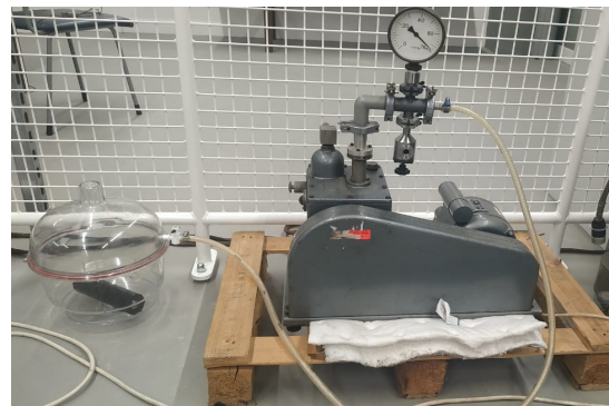
(b) Vacuum Chamber connected with Suction Pump
