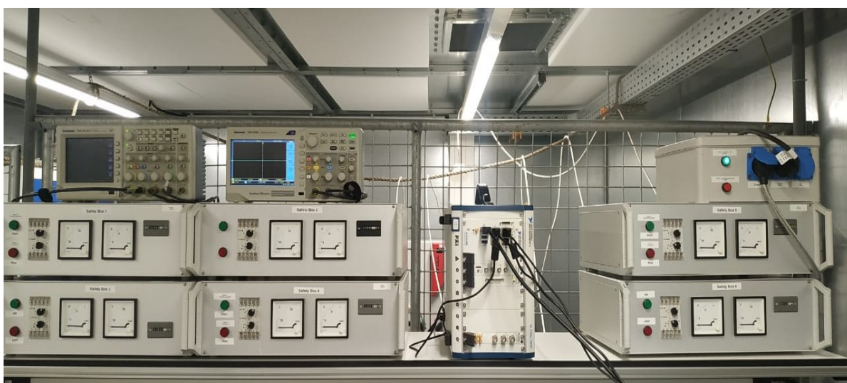
Figure 7.2: Safety Box Arrangement with PXI and Oscilloscope Setup
