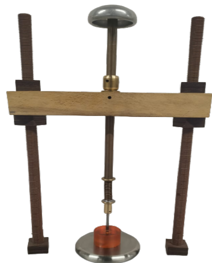
Figure 4.3: Test Cell Setup with both Electrodes and Corona Ring as used for Experiments in Chapter 6
