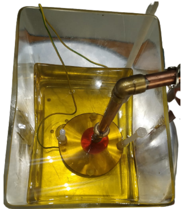
Figure 10.1: Electrode-Sample Setup for PD Measurement
