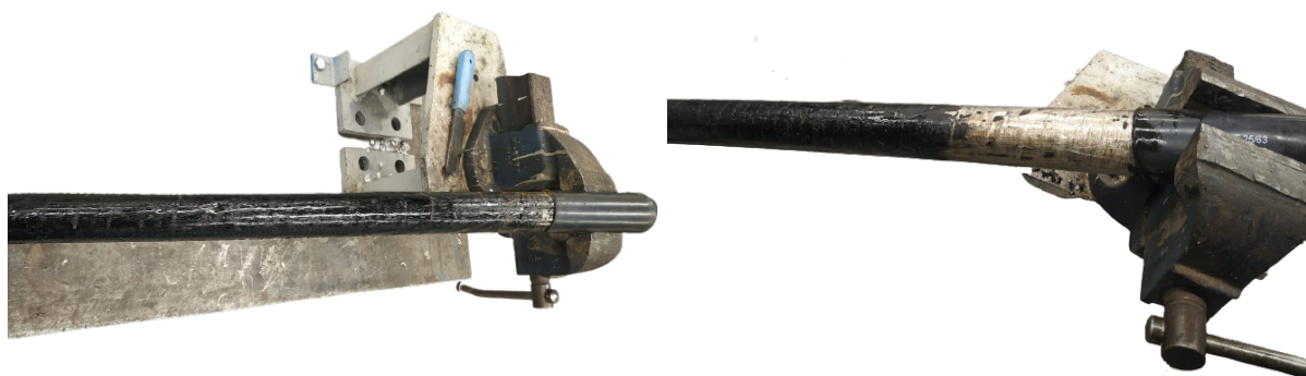
(a) Mounting the Cable without any Modifications
