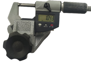
Figure 6.4: Micrometer for Measurement The cable has 3 layers of insulation, represented as the outer layer with maximum thickness, the middle layer and the inner layer with minimum thickness closest to the conductor.
