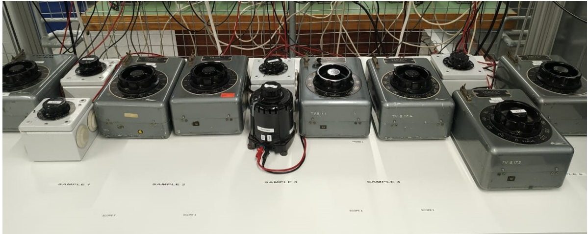
Figure 7.3: Low Voltage Side of Breakdown Test Setup
