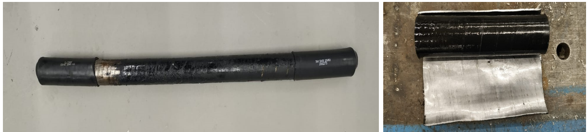
(a) Closing the terminations of the large sample with heat shrink caps
