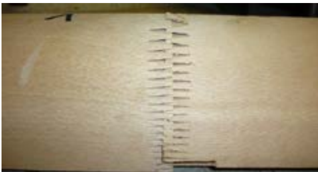
Figure 10: Half section with milled finger cuts
