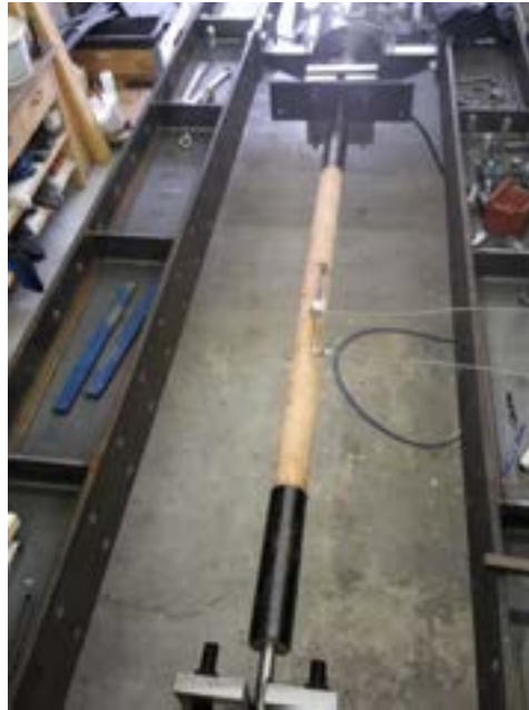
Figure 9: Test setup of a full-sized CLHS
