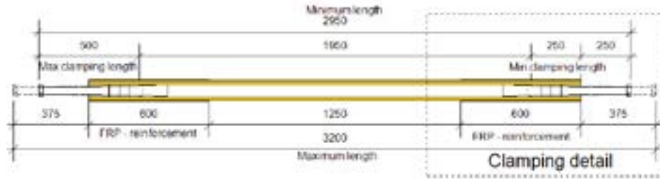
Figure 7: Longitudinal cut of the full-sized CLHS test setup including the wedge clamping construction
