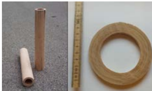
Figure 1: Beech curved laminated hollow sections CLHS prototypes (left) and related cross section with 100 mm outer diameter and 18 mm wall thickness
