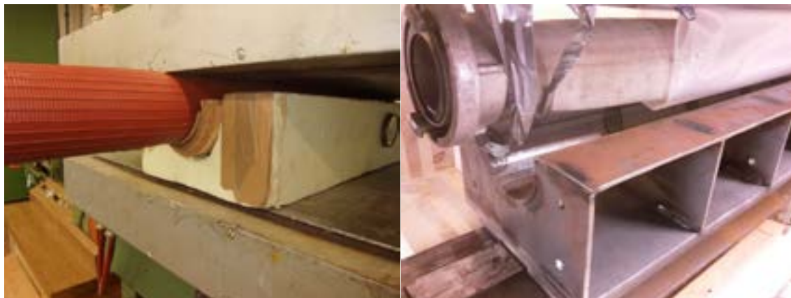
(a) Prototype of a pressing system with elastic fire hose and outer insulated cast resin form (b) Pressing system with steel moulded outer part
