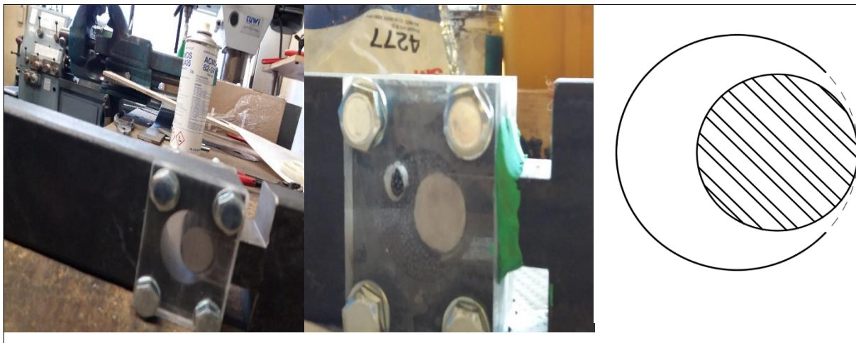
Figure 3.15: Bolt threaded part placed on the most unfavorable position inside the hole – a) in a specimen prior to injection with conventional resin, b) in a specimen prior to injection with steel reinforced resin, c) drawing of the most unfavorable position of bolt part in the hole
