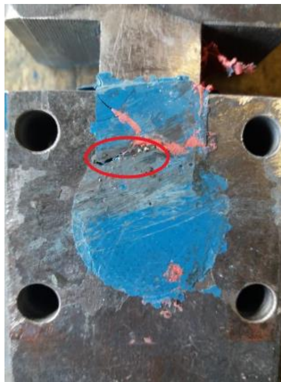
Figure 7.3: Crack due to misalignment during assembly and forced alignment by wedges of machine
