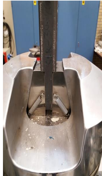
Figure 3.2 Left-Side view of lower plates (dimensions in mm), Right-Grip of the lower plate by wedges
