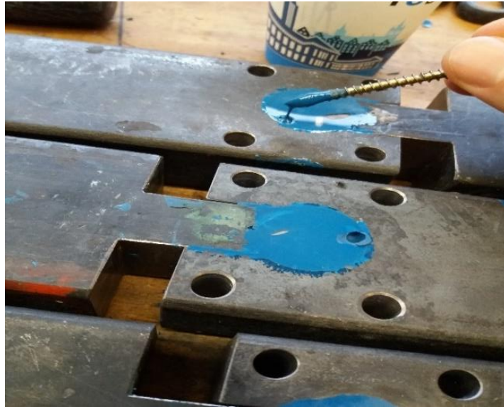
Figure 3.24: Repair of visible defects of resin part in injected specimens
