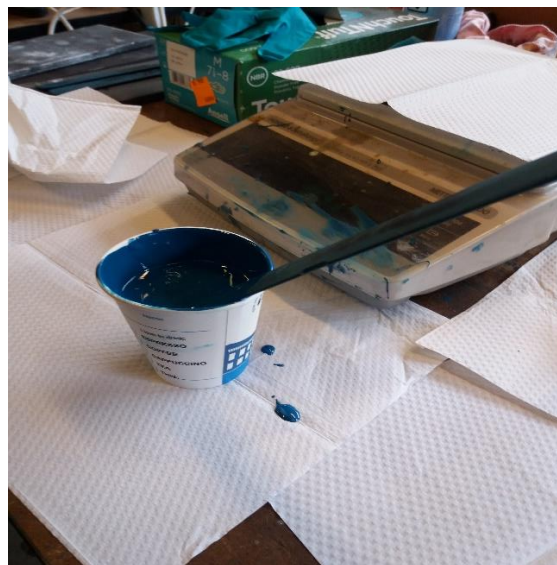
Figure 3.21: Mixing of resin SW404 and catalyst HY 5159 in ratio 8:1 using a scale and a mixing paddle
