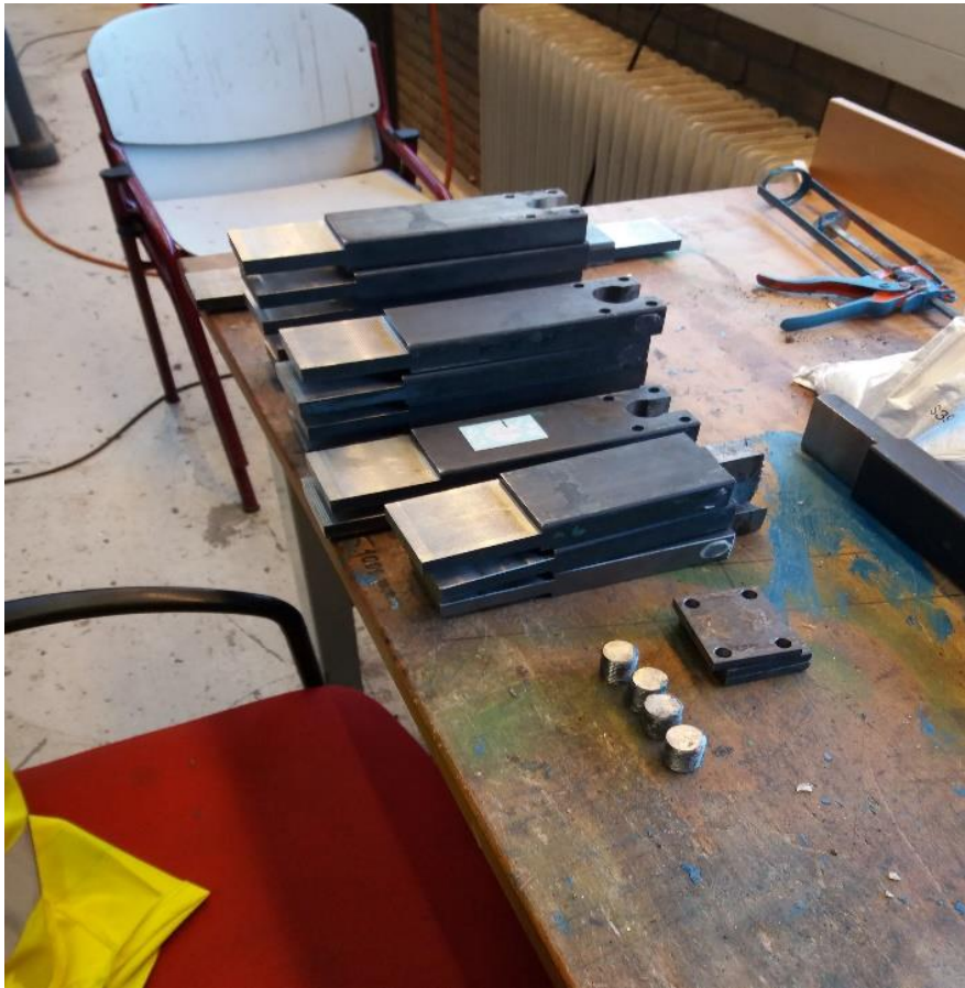
Figure 3.12: Fatigue plates used for the assembly of specimens
