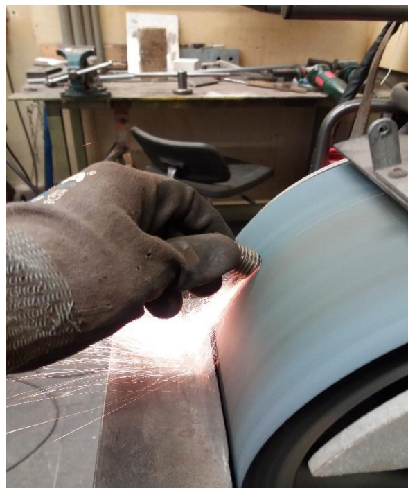
Figure 3.14: Grinding of bolt threaded part
