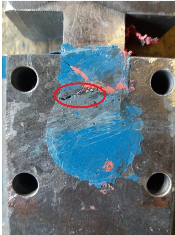
Figure 5.29: Crack due to misalignment after the position of specimen to the wedges, highlighted in red. The specimen was placed in machine fixed by wedges and removed before start of loading revealing the cracks
