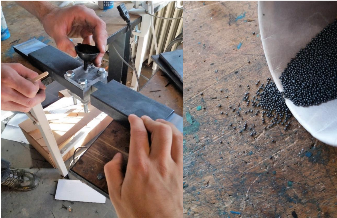
Figure 3.20: Insertion of steel shot reinforcement (left) in the hole through glass plate using funnel
