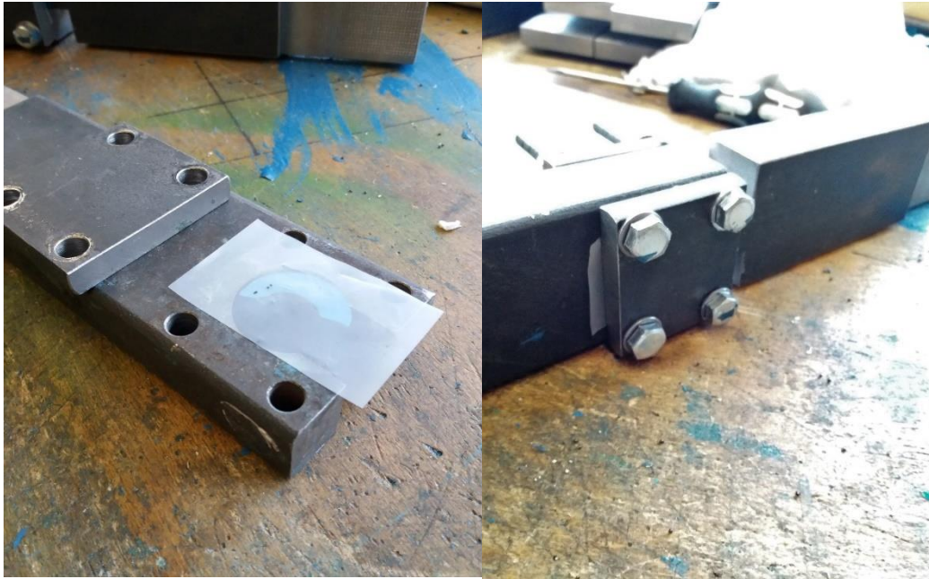
Figure 3.28: Teflon sheets placed in the expected friction surfaces (right after the dismantling of specimen, left at a specimen assembled and ready for testing)
