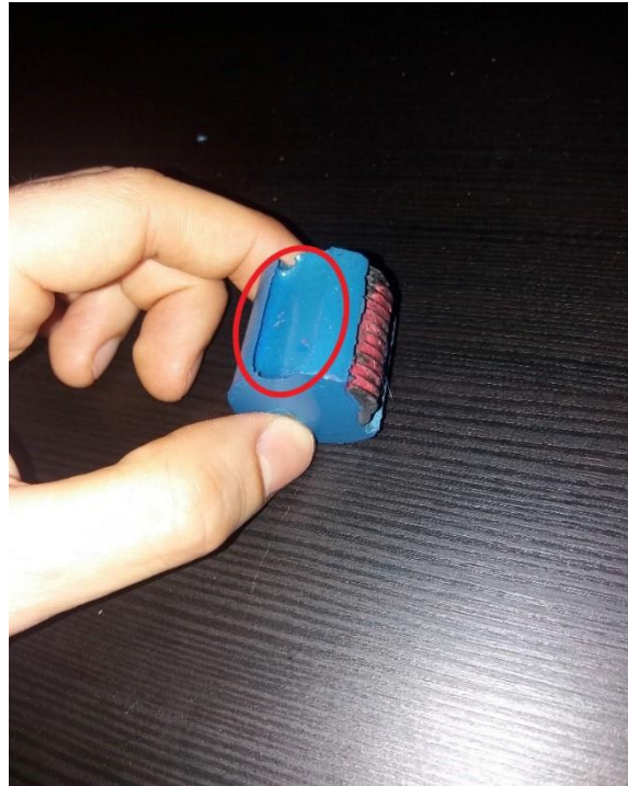
Figure 5.25: The examined in the CT scan sample with the outside missing resin part at the side
