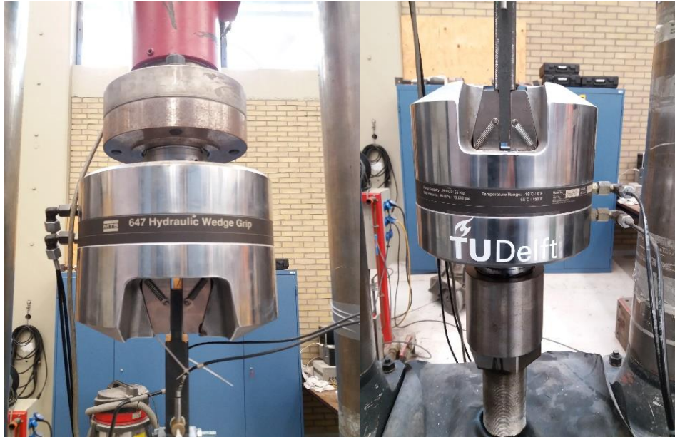
Figure 3.30: Hydraulic Wedge Grip Machine (Left-Upper wedge gripping upper plate of specimen, Right- Lower Wedge gripping lower fatigue plate of specimen)
