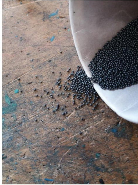
Figure 3.11: Steel shot used as the reinforcing material of steel reinforced resin used in experiments
