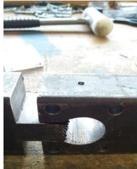
Figure 7.2: Air escape channel at the top position of steel plate to limit the air inclusions
