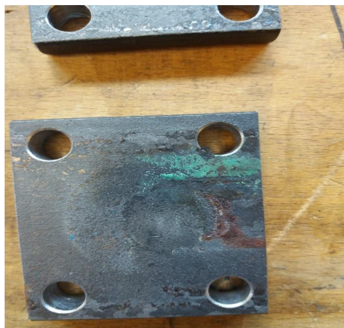
Figure 3.27: Visible effects of friction in surface of side plates after preliminary experiments
