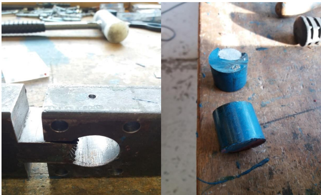
Figure 5.26: Alternative air escape path (left) and compact resin specimens after the application of the improved solution
