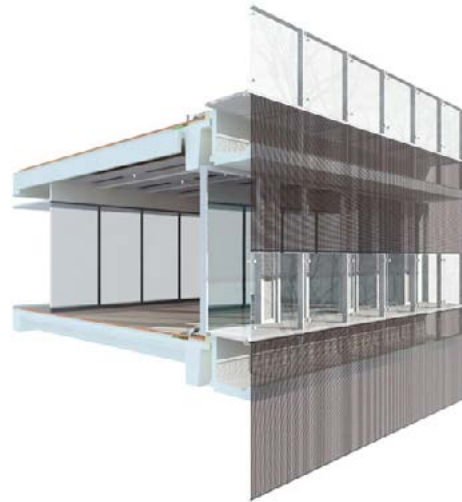
6.02 3D section of the façade principle
