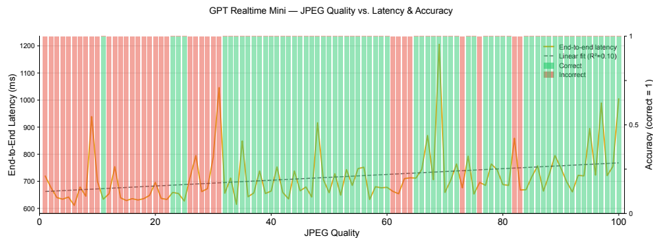
Figure A.7: JPEG quality versus total pipeline latency for gpt-realtime-mini ( R^2 = 0.10 ). A weak positive trend is visible: larger payloads at higher quality levels slightly increase latency on the streaming connection.
