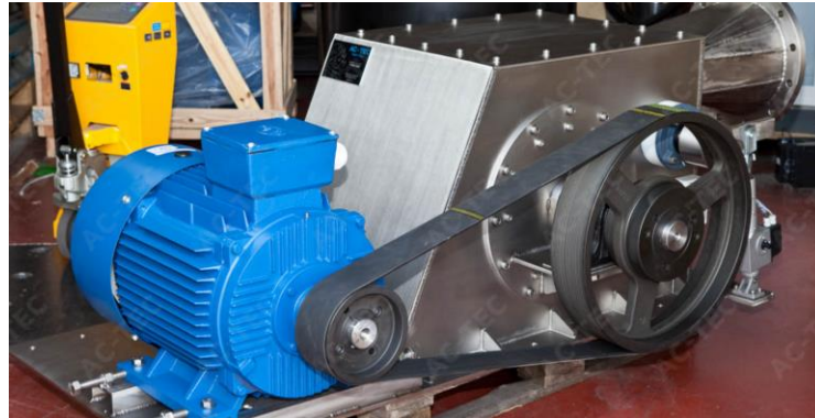
Figure E-4 A turbine coupled to its generator using a rubber belt (AC-TEC, 2015)
