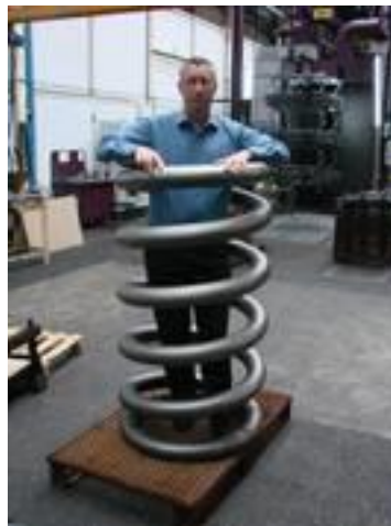
Figure B-4 An impression of a compression spring with a large wire thickness (IEN, 2016)
