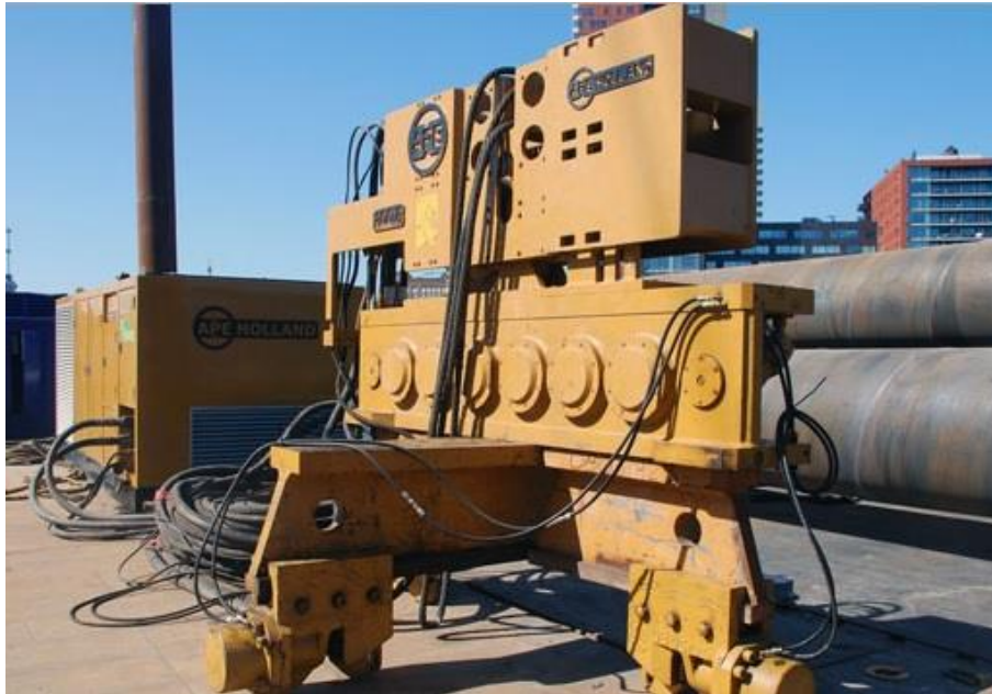
Figure D-7 Impression of the modified vibration hammer, used to install the piles with a diameter of 2400 [mm] (Gebr.deKoning, 2016)
