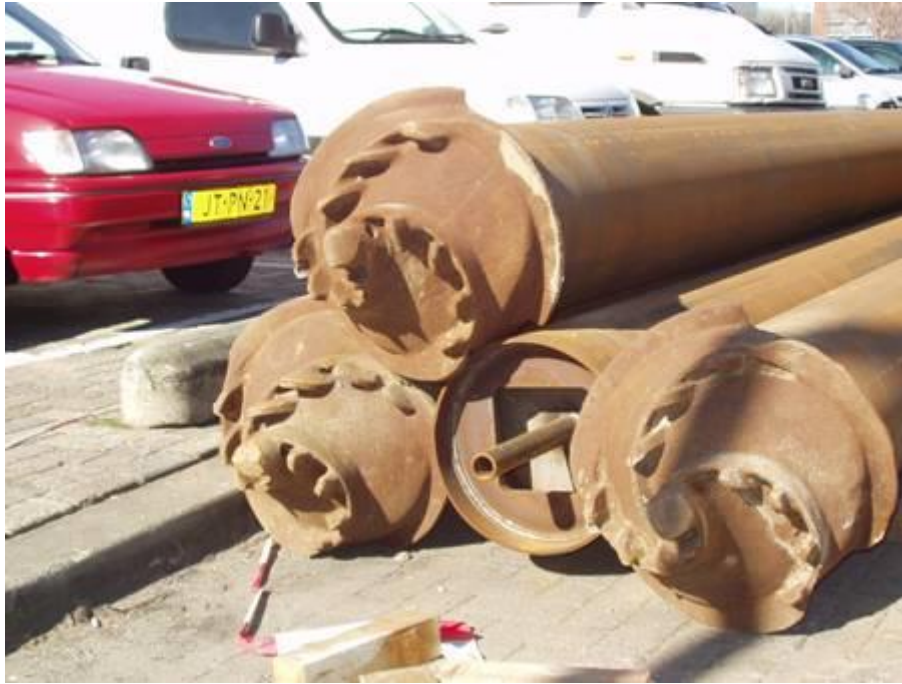
Figure D-4 Impression of multiple drill heads attached to a pile
