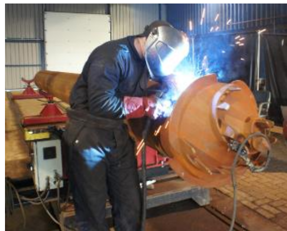
Figure 5-17 A drill tip is welded to a steel foundation pile (Solines, 2016)
