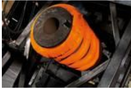
Figure B-3 A Steel bar being coiled around a spindle while red hot (IEN, 2016)
