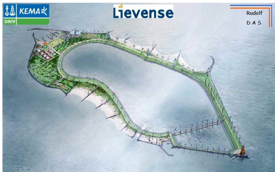
Figure A-8 Artist impression of an inverse off shore pump accumulation station ( Boer, 2007)
