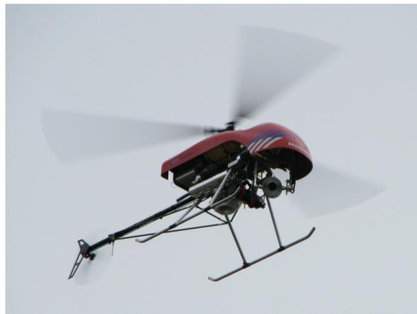
**Figure 1-1:** RH2 ‘Stern’ UAV helicopter designed and manufactured by Delft Dynamics B.V. is one of many UAVs introduced recently in the civilian market (Delft Dynamics, 2006)
