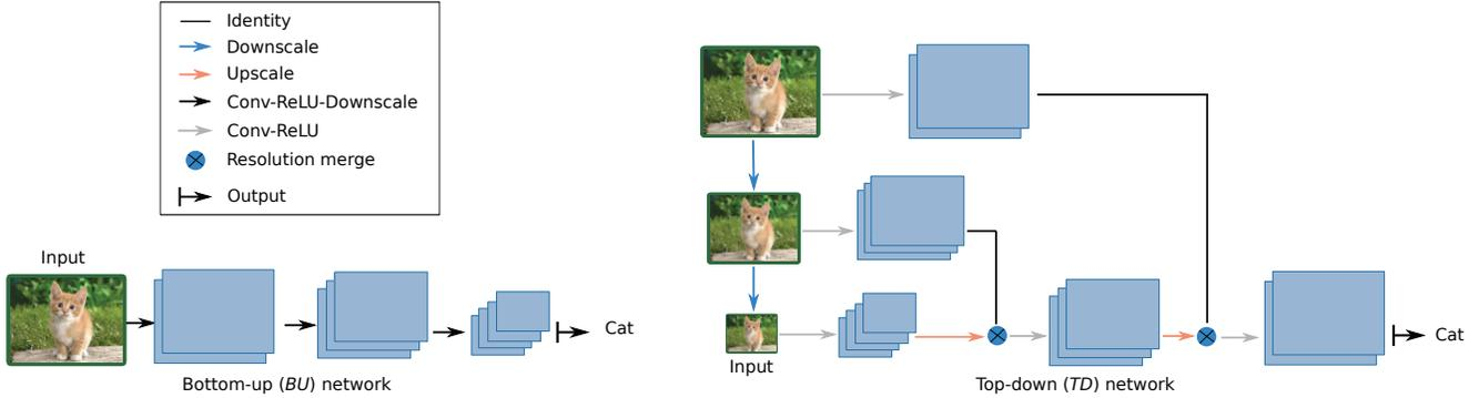
Figure 2. **Left:** The bottom-up (*BU*) baseline network. Feature maps decrease in spatial resolution with network depth. **Right:** The proposed top-down (*TD*) network. The *TD* model reverses the feature extraction pathway of the baseline network. It employs three inputs from highest to lowest scale, starts processing from the lowest resolution and progressively adds high resolution information.
