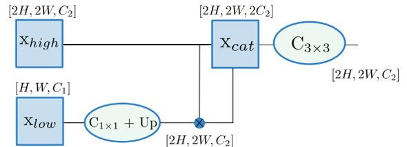
Figure 3. Merging low and high-frequency feature maps: we use a  $1 \times 1$  convolution followed by an element-wise addition; this information is concatenated with the high-resolution input and followed by a  $3 \times 3$  convolution that expands the receptive field size.
