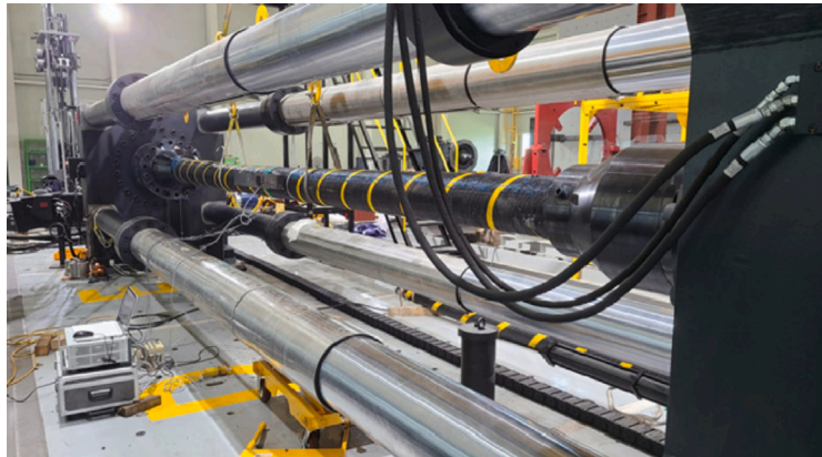
Fig. 7. Tension test facility [41].
