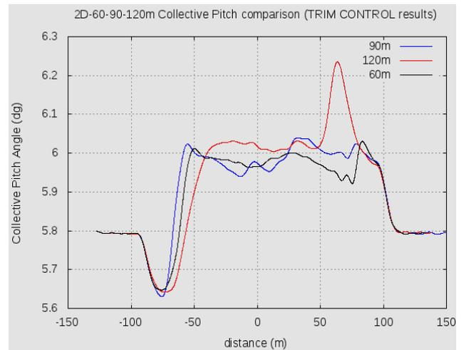
Figure 17 Collective pitch comparison for wake crossings at different heights
