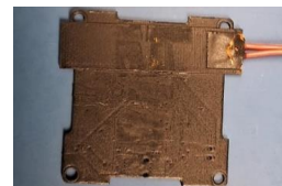
Figure 4. PCB with LabIR paint of known emissivity ( \epsilon_{IR} = 0.8 ) for Test 2
