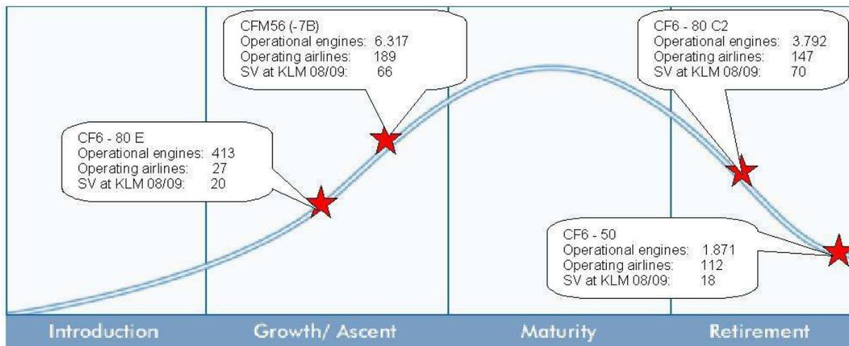
Fig. 2 The main overhauled Engine types located on the product life cycle
