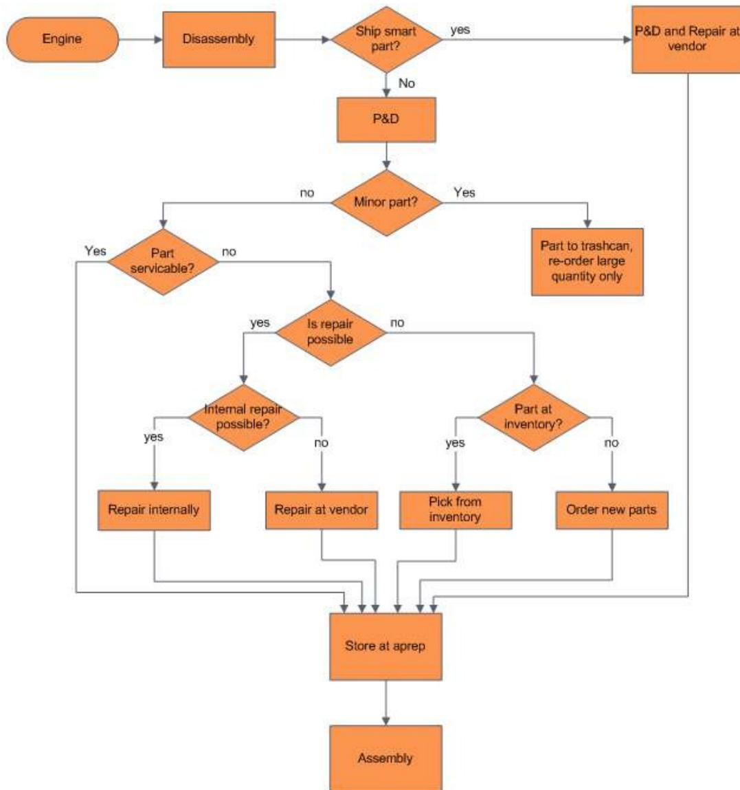
Fig. 7 general material flow during engine overhaul
