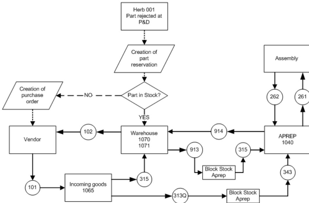
Fig. 10 Physical flow diagram Rejected herb 1 parts
