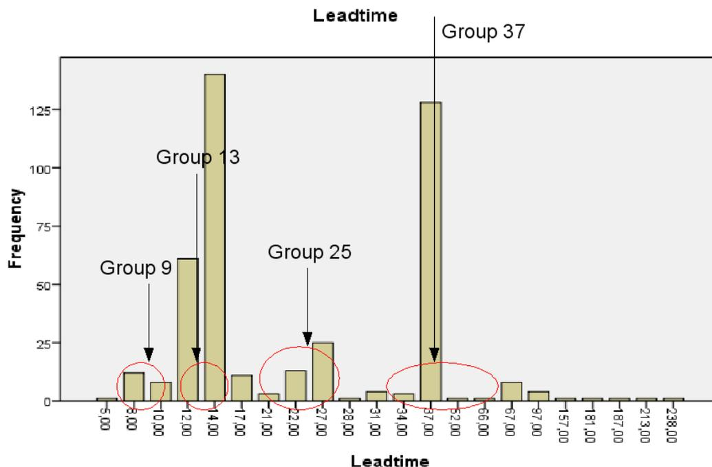
Fig. 30 Frequency of material numbers per lead time and related material grouping
