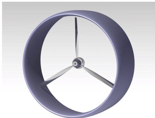
Figure 2.3: Propeller and shroud layout
