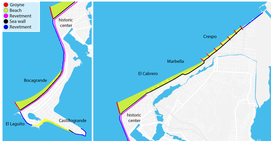
Figure 5.9: Overview of alternative 'Two groynes'
