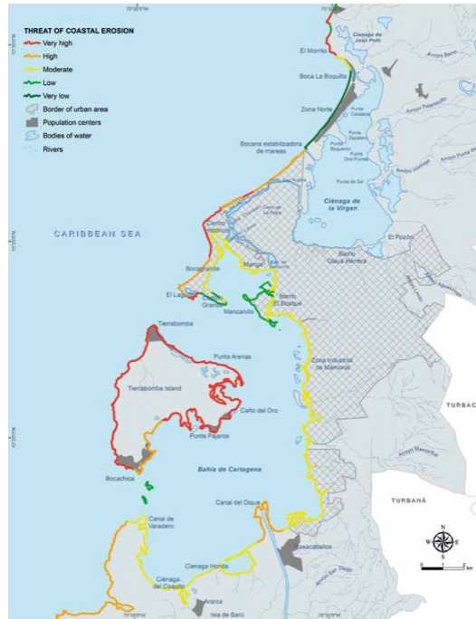
Figure 2.13: Threat of coastal erosion (CDKN et al., 2014)
