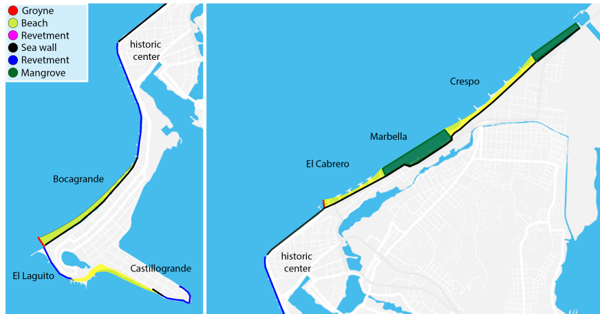
Figure 5.10: Alternative using mangrove swamp
