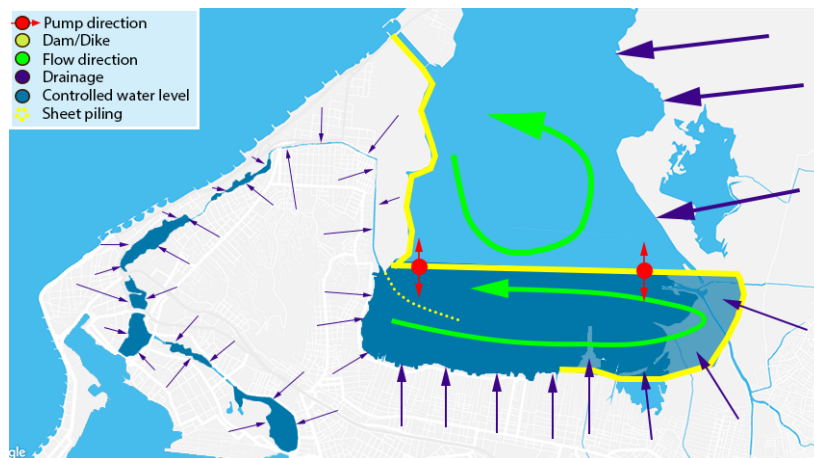
Figure 5.3: Ciénaga alternative 2 - Controlling the urban shore
