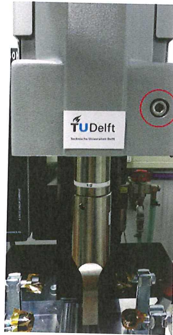
Figure 2-12 | Front view USW machine, highlighted bolt is used to loosen the complete welding train
