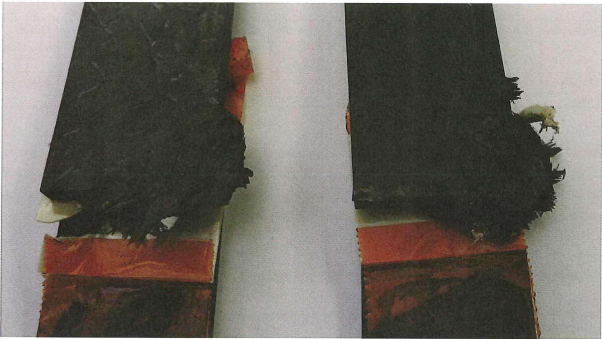
Figure 3-6 | Melting on 100% travel chopped to chopped fibre welded sample, showing extensive deconsolidation mostly in the top sample, showing samples #45 and #46 (appendix B)
