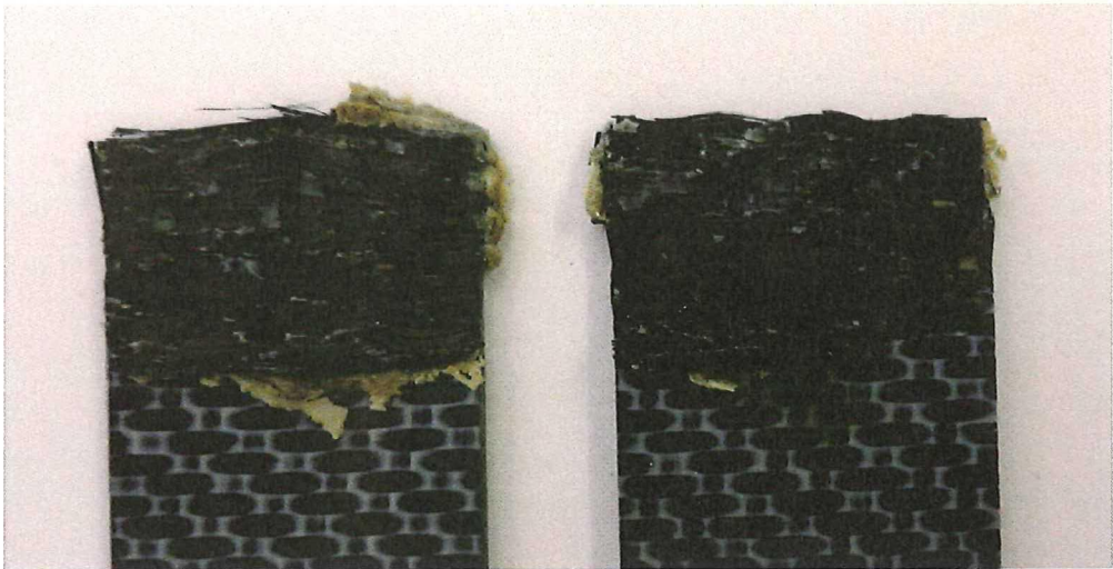
Figure 5-27 | Fracture surfaces of sample #125 (appendix B), welded with pre-attached ED
