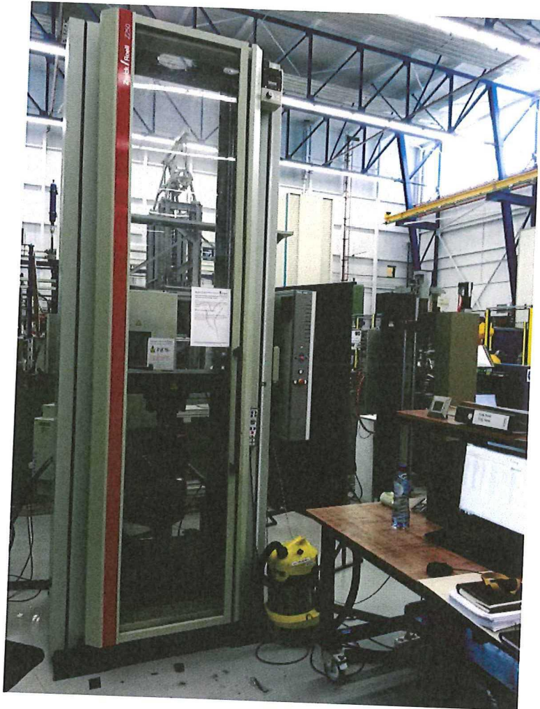
Figure 2-17 | Zwick 250 kN universal testing machine used for static lap shear strength determination
