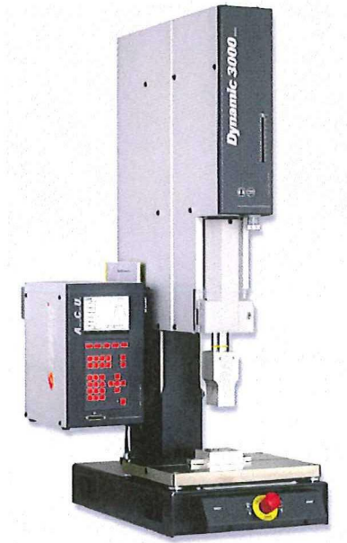
Figure 2-9 | Rinco Dynamic 3000 ultrasonic welder equipped with an Advanced Control Unit
