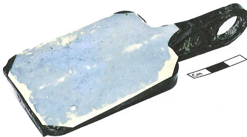
Figure 2-8 | Chopped fibre hinge with extra layer PEEK attached using the same film stacking process
