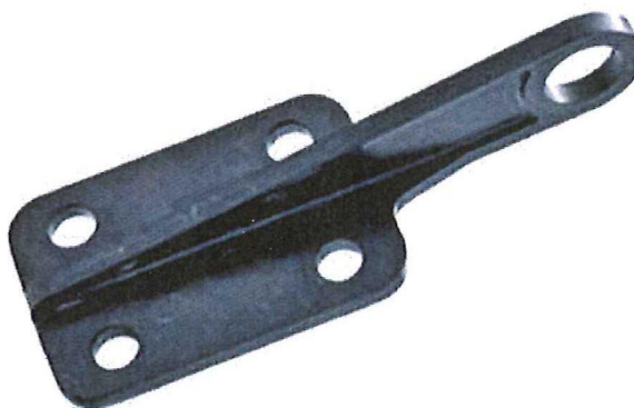
Figure 1-2 | Schematic view of the TPC helicopter door hinge (left) and actual view of the door hinge produced of recycled CF/PEEK (right) by FHWN [8], [9]
