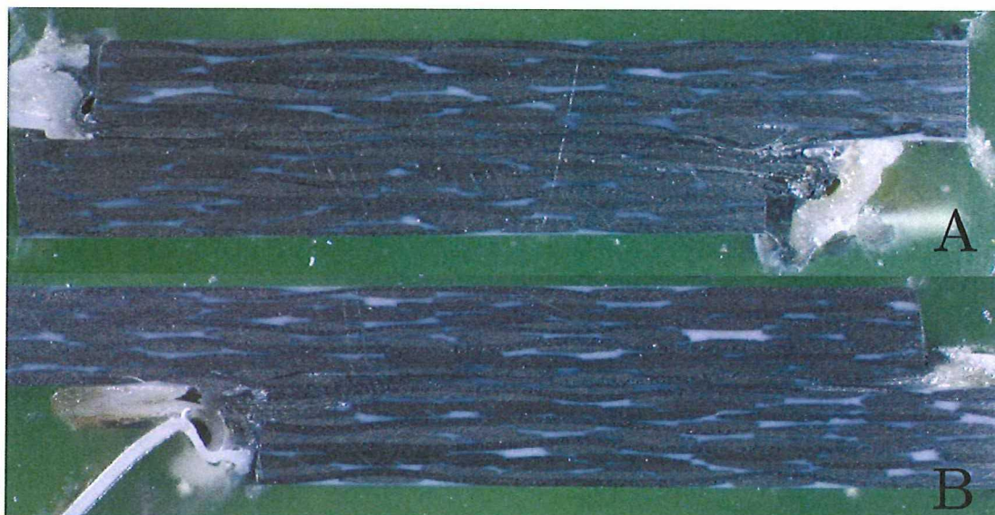
Figure 3-4 | Sample A (#09, appendix B) cross section of a Toho Tenax weave – weave weld using 300 [N] welding force, Sample B (#17, appendix B) cross section of a Toho Tenax weave – weave weld using 1000 [N] welding force, 1.25x magnified
