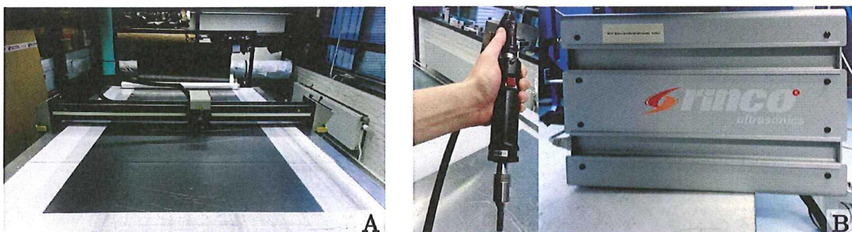
Figure 2-3 | DASML – A) Automatic sheet cutting machine, B) Ultrasonic hand plunge welder
