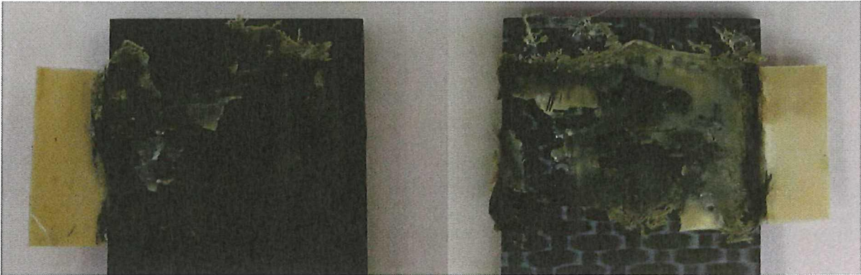
Figure 5-22 | Typical fracture surface for the welding of weave (Ten Cate 90 [°]) to chopped fibres using the dedicated area sized ED welding (sample #117, appendix B)
