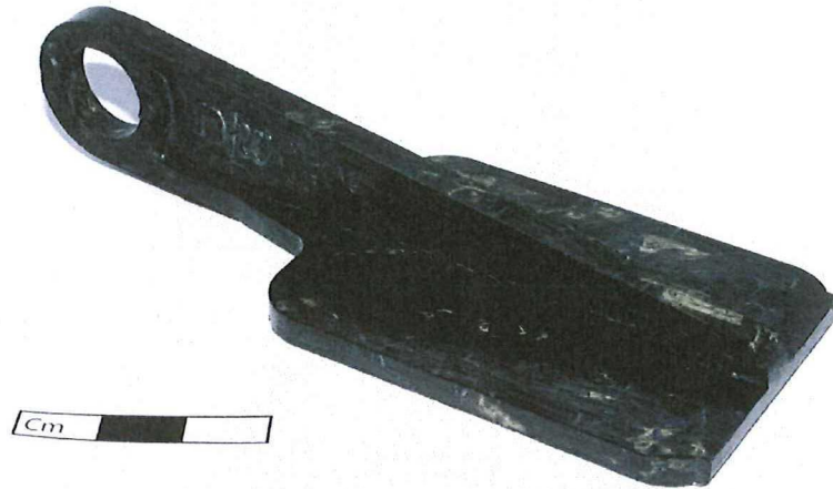
Figure 2-2 | Newly produced hinge, without holes in the bottom plate, using Toho Tenax CF/PEEK chopped fibre material
