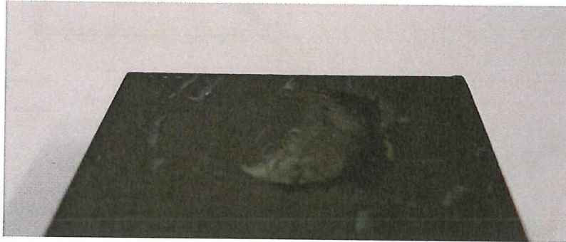
Figure 3-7 | Surface damage as a result of an energy controlled welding experiment, delivering 500 [Ws] of energy with the Ø 10 [mm] cylindrical sonotrode, using a 300 [N] welding force, sample #94 (appendix B)
