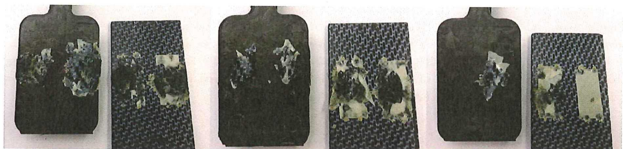
Figure 6-16 | Fracture surfaces of welded hinges 8 (left), 9 (middle) and a one side welded hinge (right), first and second spot welds for the hinges are, L=Left, R=Right: 8 (1: R, 2: L), 9 (1: L, 2: R) and only the left one for the last hinge
