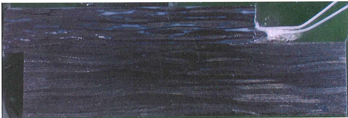
Figure 3-9 | Sample #55 (appendix B) section of a continuous weave (top sample) to a chopped fibre (bottom sample) weld, 1.25x magnified
