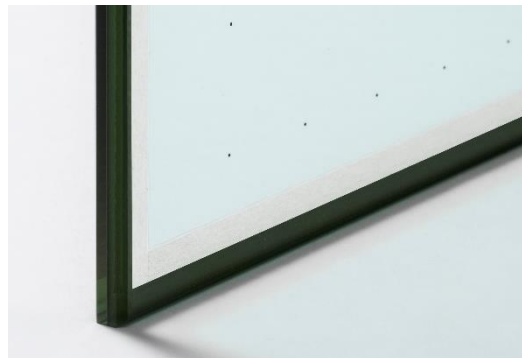
Image 14 - VIG panel. 2 layers of 3mm glass with cavity of 0,1mm. Photo: AGC
