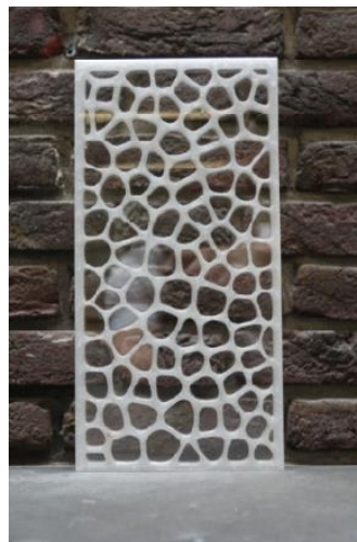
Image 2 - 8 mm core thickness. 1 mm thin glass (Neeskens, 2018)
