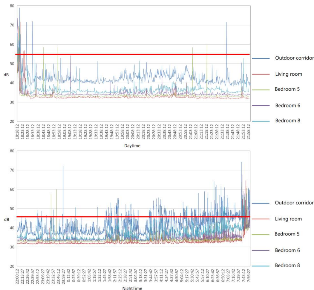
Figure 16. Acoustic on-site measurement results.
