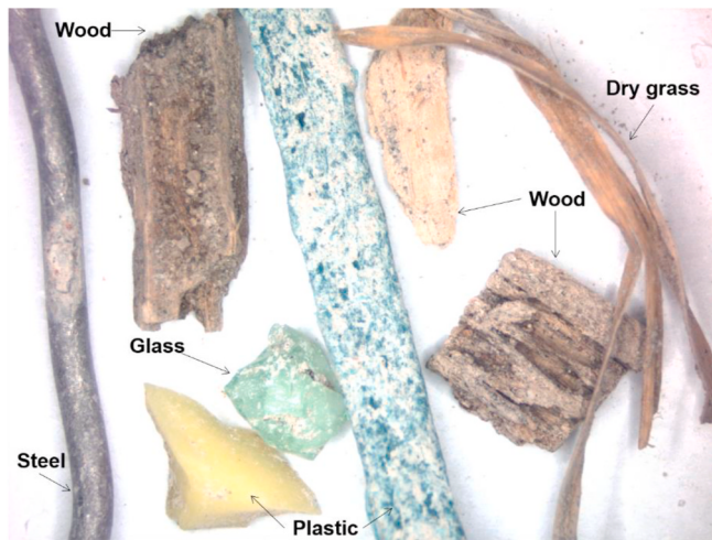
Fig. 11. Stereomicrograph of different contaminants in fRCA.
