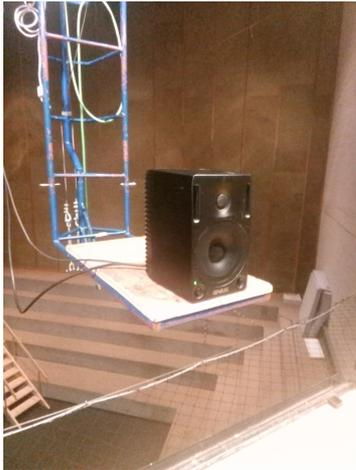
(a) Genelec 1029A positioned on the crane at the *cube* facility in Struer, Denmark. The loudspeaker is rotated to perform directivity measurements.
