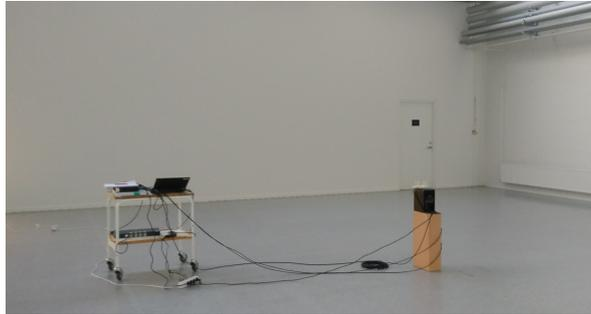
Figure 4.11: Genelec 1029A positioned in front of a large single wall. The microphone array is approximately one meter from the floor.
