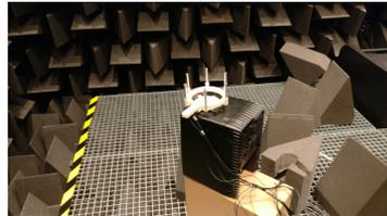
(b) An uniform circular microphone array with six microphones is placed on top of the loudspeaker. The direct path impulse response for all microphones in the array.
