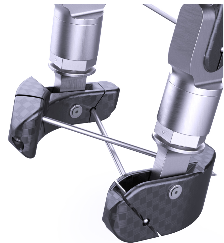
Figure 59: rotation axis incorporated within the design
