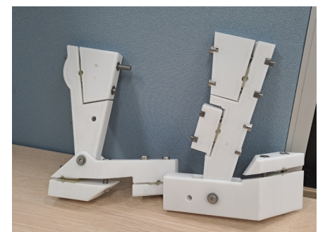
Figure 49: prototype printed out of PC
