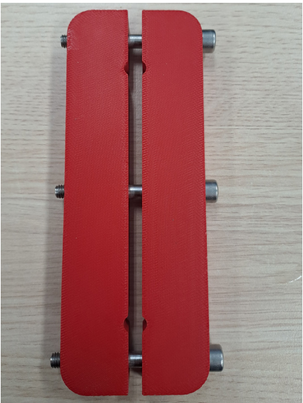
Figure 32: Standardized clamps for the tibia pins
