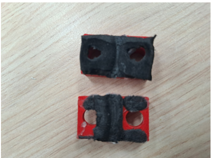
Figure 34: Dent on the inside of the clamp
