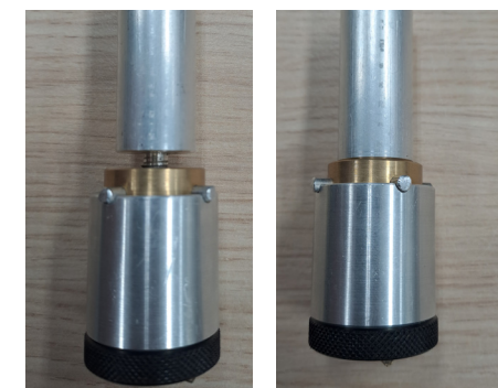
Figure 40: prototypes of distraction mechanism without distraction (left) and with distraction (right)
