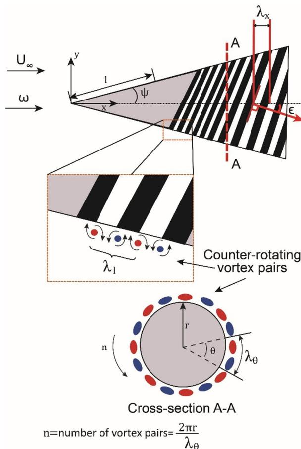
Fig. 2 Schematic representation of the flow field depicting typical footprints of the spiral vortices on the surface temperature along with the definitions of wavelength components ( $\lambda_l, \lambda_x, \lambda_\theta$ ), number of spiral vortices ( $n$ ), and spiral vortex angle ( $\epsilon$ ). Effects of the surface curvature on the fringes is not shown for simplicity
