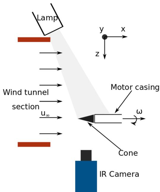
Fig. 1 Schematic of the experimental setup (top view)
