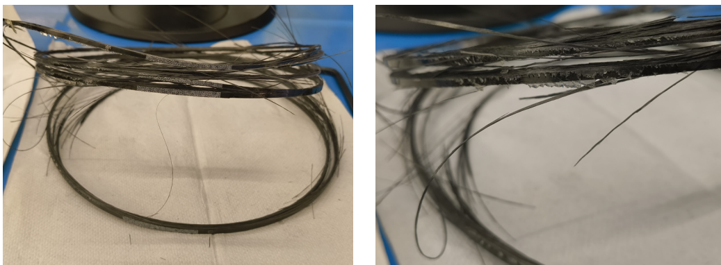
Figure 6.22: Specimen 7 Fatigue Failure after 75 cycles (240 kN, R = 0.1 , 0.42 Hz)
