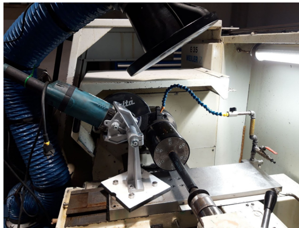
(b) Specimen Cutting with a PCD Tool on the Lathe
