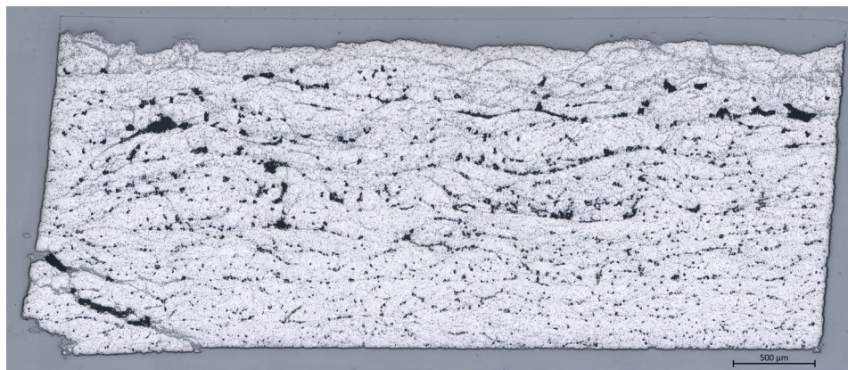
Figure 5.15: Specimen Cross-section (white - fibres, grey - matrix, black -voids)
