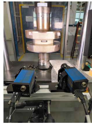
(b) Setup B: 4 MP Cameras with 50 mm Lenses
