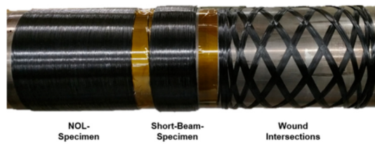
Figure 5.12: Filament Winding of Hoop and Helical Layers 1
