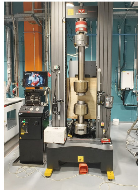
(b) Instron 5985 Electromechanical Test Bench (250 kN)
