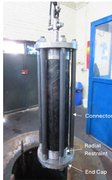
Figure 3.3: Hydrostatic Pressure Test Setup [27]
