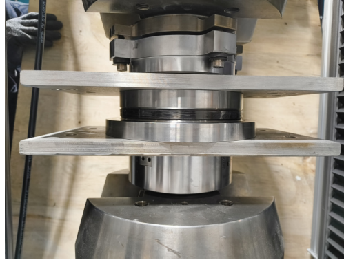
Figure A.5: Test Setup with 'Extended' Compression Plates
