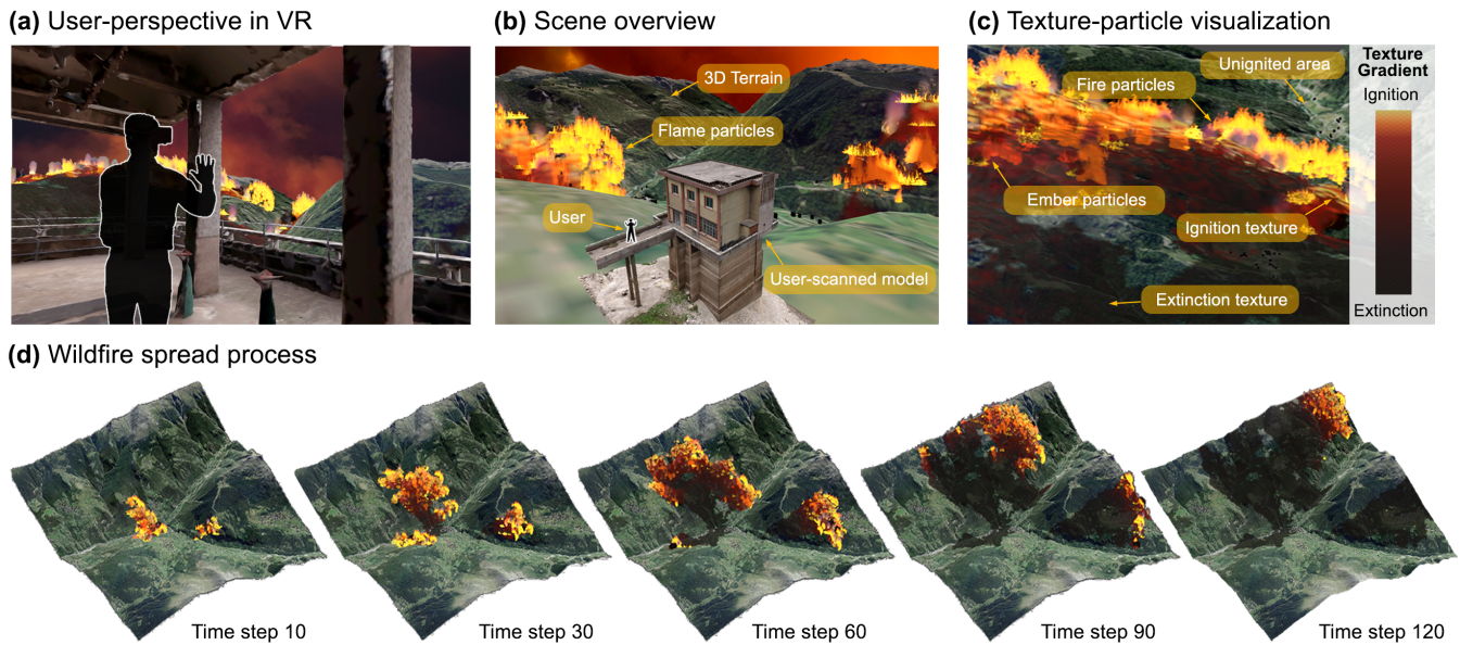
Figure 5: (a) Training takes place from a first-person perspective in VR. (b) A third-person view shows the relations between the user, the scanned model, and the surroundings in the wildfire scene. (c) Wildfire visualization combines particles (flames, embers) with terrain textures indicating different fire states. (d) The wildfire spread process is simulated over time.
