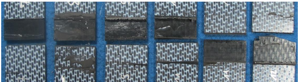
Figure 8.11: Fracture pattern SLS-APP- hotwet-75°C bonded with a) EP_1, b) EP_2 and c) PU
