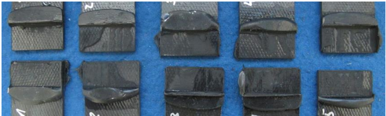
Figure 8.13: Fracture pattern CF-PEEK-SLS-APP- dry-RT- bonded with a) EP_1, b) EP_2 and c) PU
