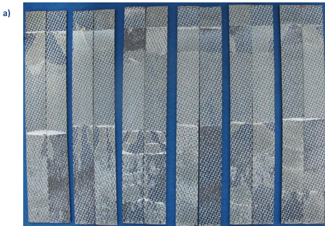
Figure 8.6: Fracture pattern DCB-APP- dry-RT- bonded with a) EP_1, b) EP_2 and c) PU
