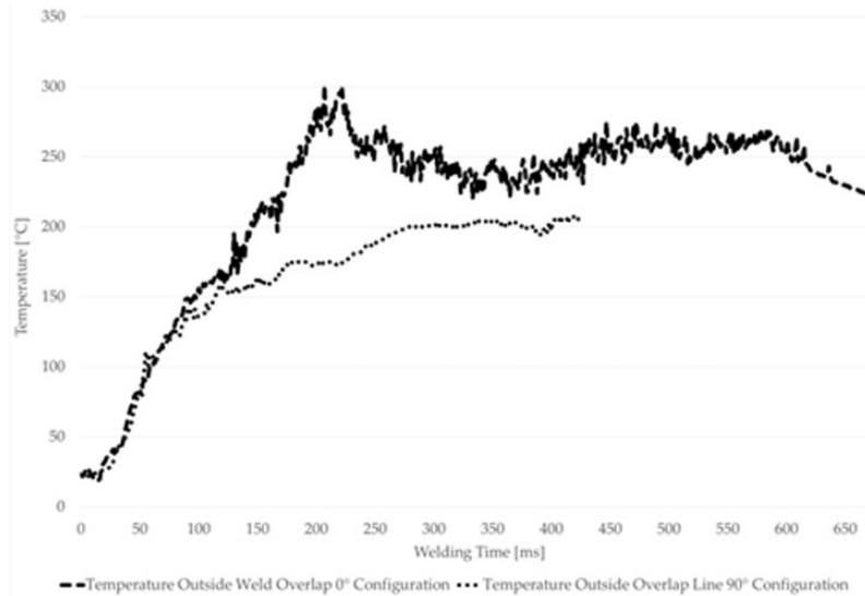
Figure 9. Temperature measurement outside the weld overlap on top of upper adherend for configuration 0° sample (solid line) and configuration 90° (dotted line). Welding performed with 86.3 \mu\text{m} amplitude, 1000 N weld force and 0.16 mm vertical displacement.
