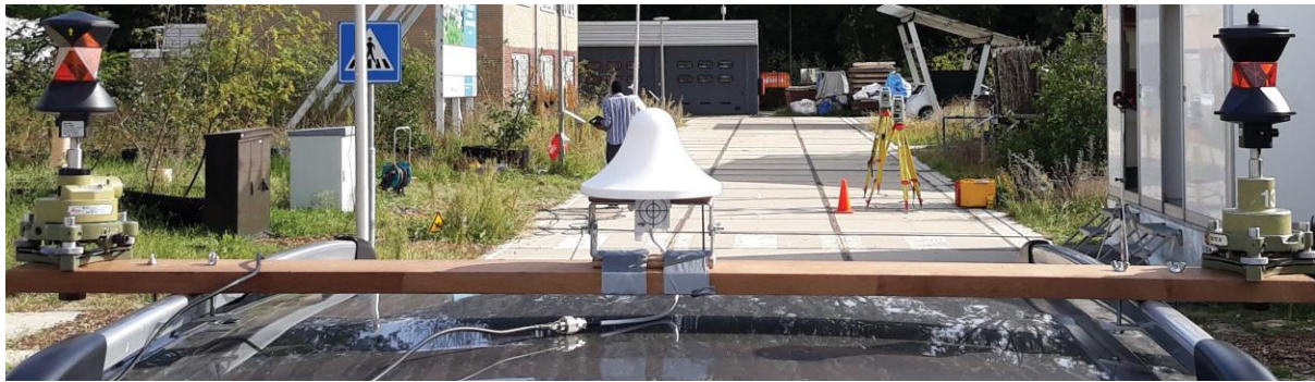
FIGURE 5. Receiver antenna mounted on the roof of a car. Two 360° prisms are used to determine the receiver ground-truth positions at the millimeter level, by means of land surveying total stations (placed on the yellow tripods in the distance).
