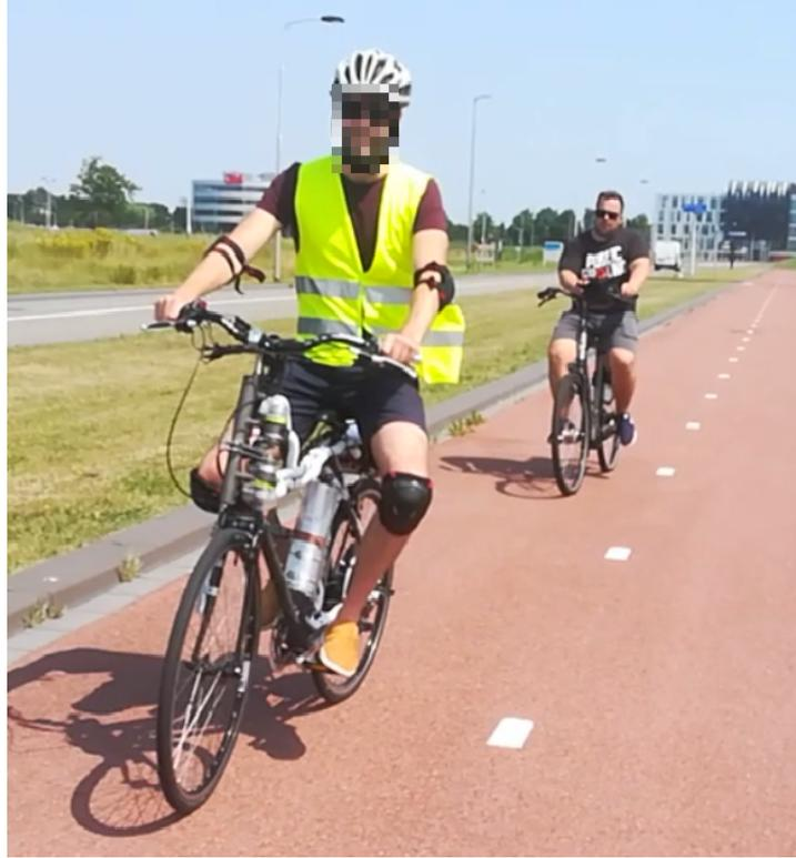
Figure 4.1: Experimental trial performed across Heertjeslaan cycling path of TU Delft; Experiment coordinator cycling behind the steer-by-wire bicycle perturbing the subject through the mobile interface.
