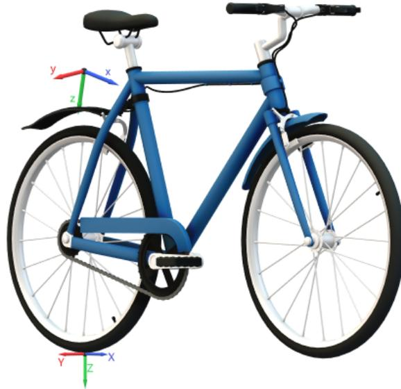
Figure A.1: Bicycle with body fixed sensor axis x-y-z (B) and global axis XYZ (G).
