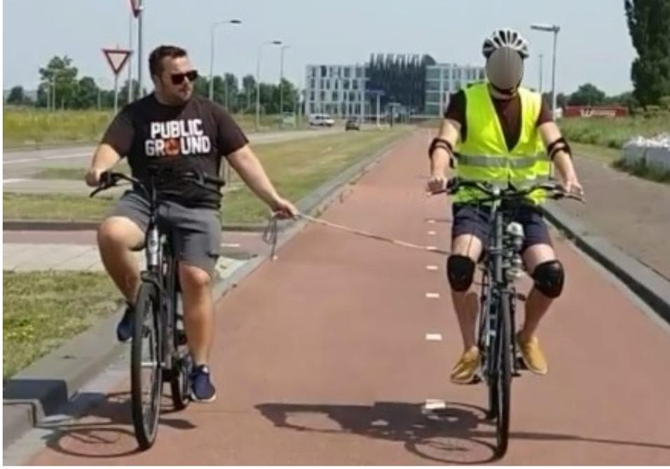
Figure 2.2: Experimental trial performed across Heertjeslaan cycling path of TU Delft; Experiment coordinator cycling next to steer-by-wire bicycle while pulling laterally the subject with a rope.
