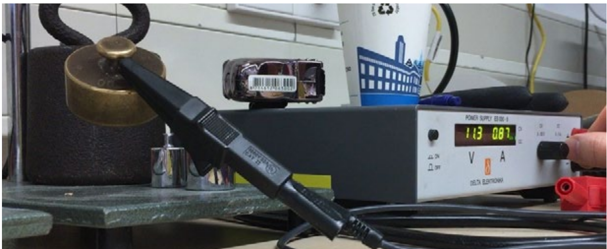
Figure 9 Lifting weight using SMA wire
