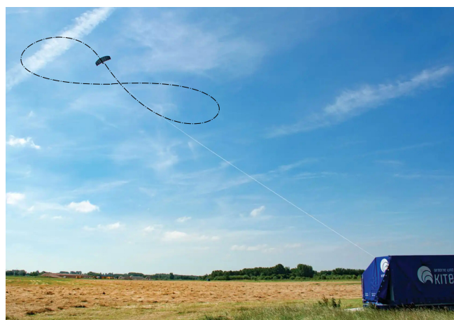
(b) The Falcon harvesting electricity in former naval airbase Valkenburg [38] with an added figure of eight illustration.
