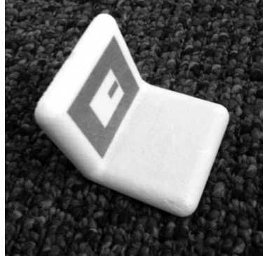
Figure 39 Coloured 3D printed object with embedded marker.
