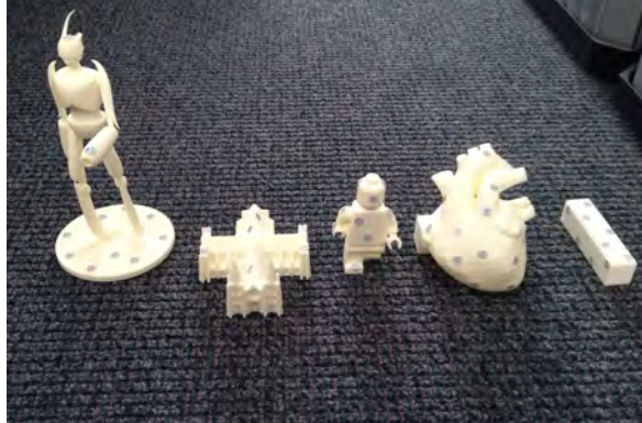
Figure 49 Test objects equipped with retro reflective markers.
