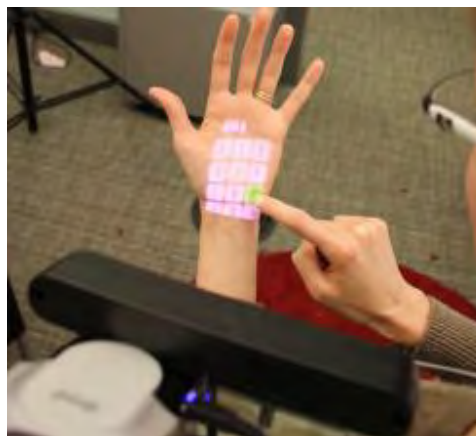
Figure 14 Wearable projector with hand tracking (Harrison et al., 2011).
