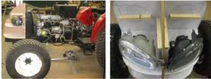
Figure 23 Left: elongated tractor chassis that was reverse engineered, right: wooden section model of the body, to select and fit the car headlights into the new shape.
