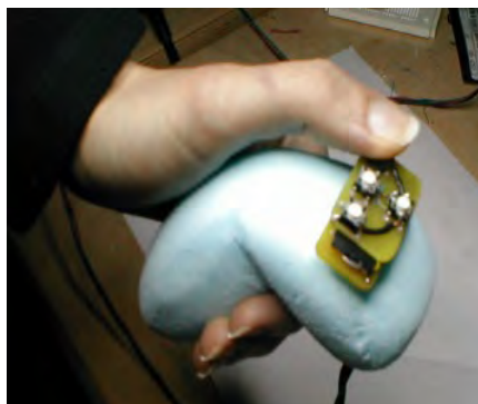
Figure 19 Mock-up equipped with wireless switches that can be relocated to explore usability (Lee et al., 2004).
