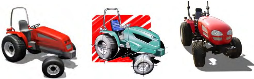
Figure 22 Design stages of the tractor design. Left: early 3D model, middle: sketched concept, right: picture of the null series.
