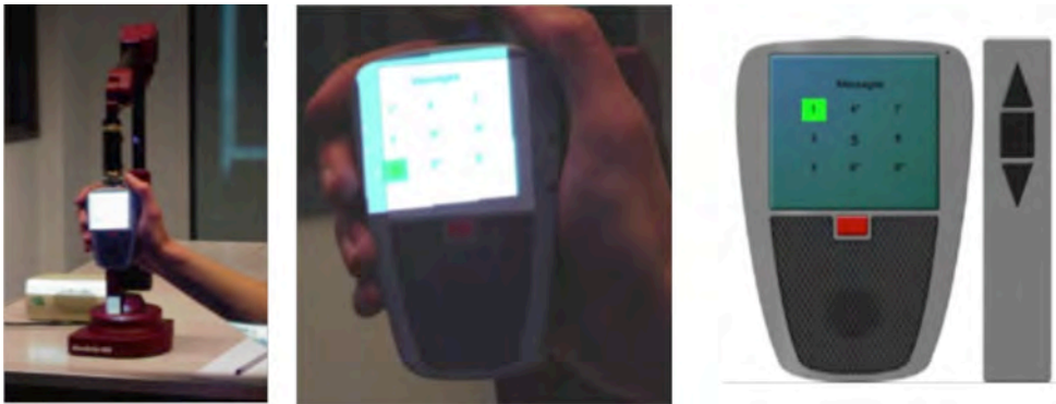
Figure 57 Voice recorder system (left), projection (middle) and 2D screen prototype (right).
