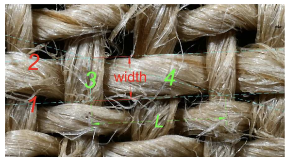
Figure 4. The geometries used to measure yarn width (lines 1, 2) and twist (lines 3, 4 and segment L).
