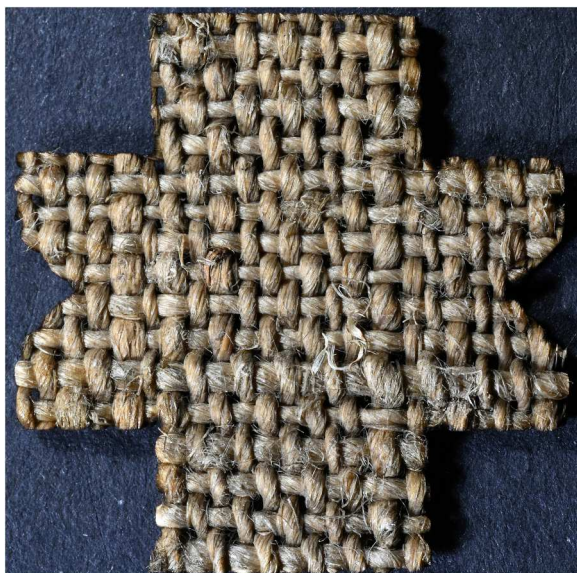
Figure 2. The image of one of the laser-cut samples (n. 2 in Table 1), with the indentations in the weft direction.
