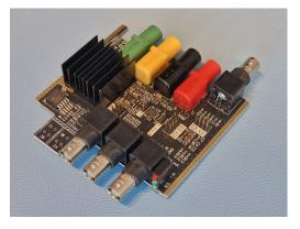
Figure 3.17: Custom PCB without enclosure components.
