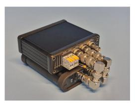
Figure 3.18: PEH emulator connected to Joulescope for power measurement.
