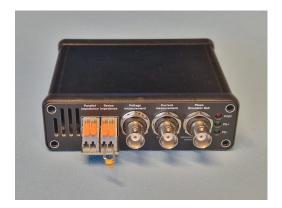
Figure 3.15: Front panel of the PEH emulator.
