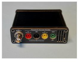
Figure 3.16: Rear panel of the PEH emulator
