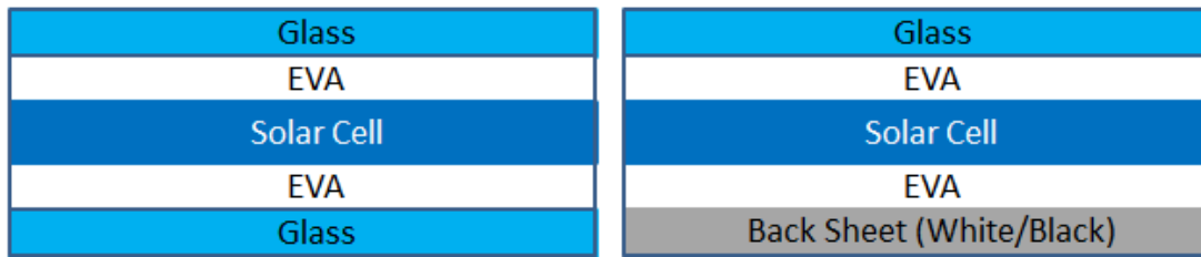
Figure 22: Configuration of (a) the glass-glass module and (b) module with back sheet.
