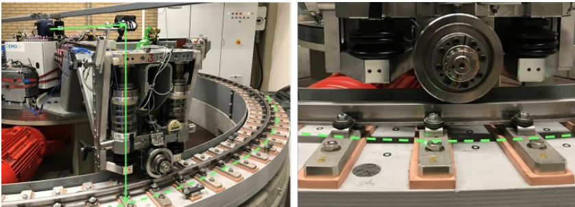
Figure 1.2: LDV on the moving platform of the TU Delft V-Track test rig.
