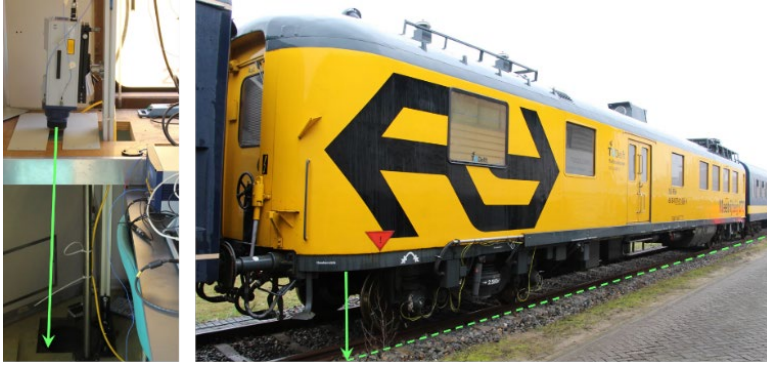
Figure 1.3: Train-borne LDV on the CTO measurement train of TU Delft.
