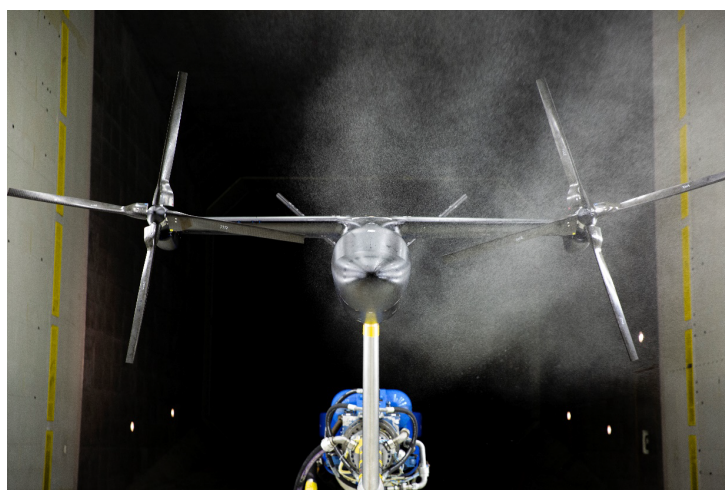
(b) HFSB streamtube on a tiltrotor aircraft model
