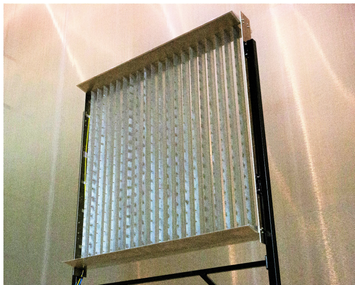
(a) 400-nozzle, 3 \times 3 \text{ m}^2 HFSB seeding generator
