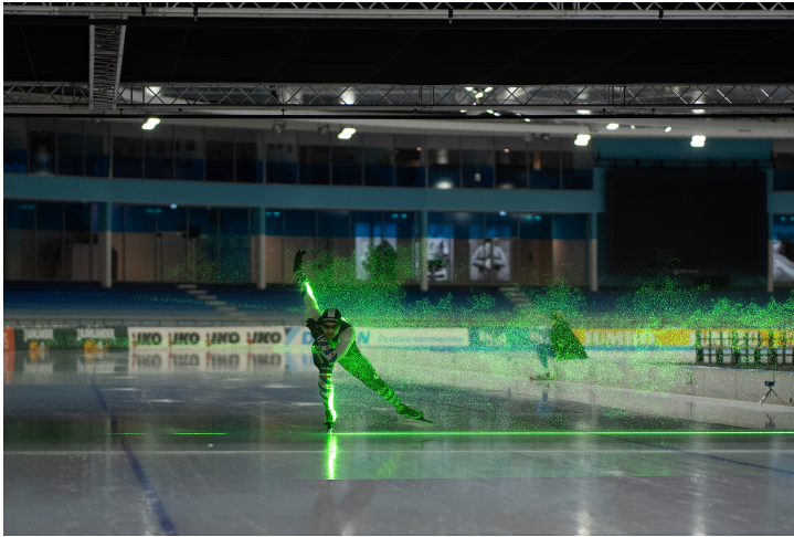
Figure 2.10: On-site aerodynamic study of a speed skater with HFSB tracers for stereoscopic PIV measurements. Image reproduced from TU Delft (2021) .
