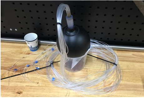
(a) Model preparation: installing the pressure tap tubing.
