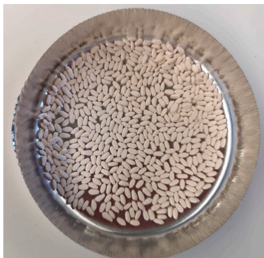
Fig. 1. Printed zeolite granules (after sintering at 950 °C).
