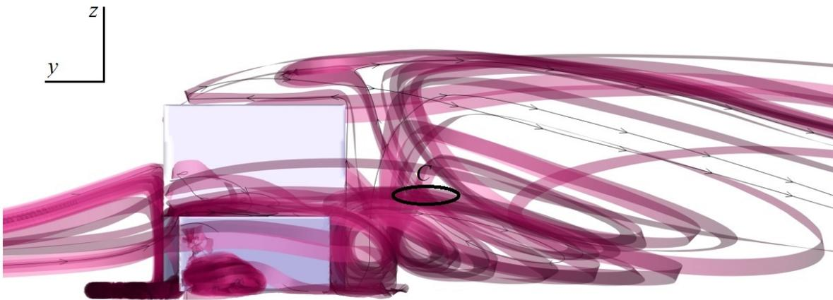
**Figure 7.11:** Rear-view of the baseline ship (*LPD2-Model2*) for a R105 relative wind angle and 29 kts wind speed (cross facing port procedure).
