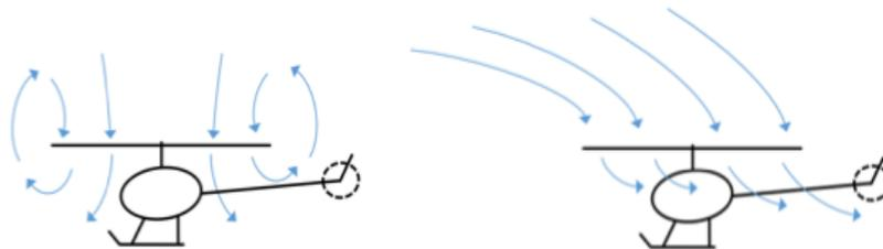
**Figure 2.4:** Left: inefficient rotor due to recirculation of disturbed air - Right: efficient rotor due to translational lift.
