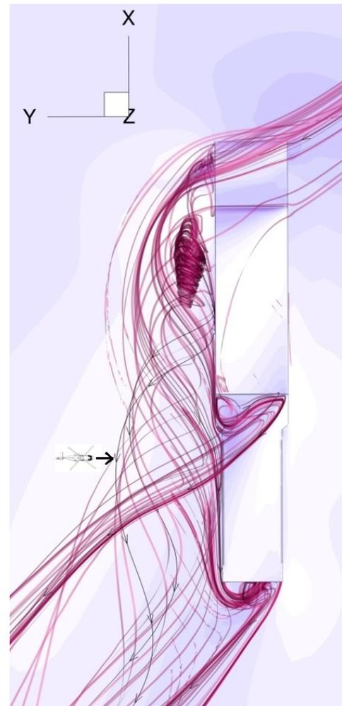
**Figure 5.16:** Top view: High pilot workload leeward of the flight deck, for cross winds.
