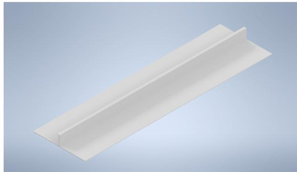
Figure 11.4: Plate-stiffener used in experiment
