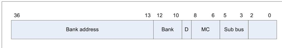
Figure 4.3: Composition of a virtual memory address
