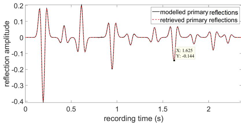
**Figure 6-2:** The obtained subsurface primaries (red dashed line) and the modelled reflectivity (black solid line) convolved with the 20 Hz Ricker wavelet as a function of two-way travel time
