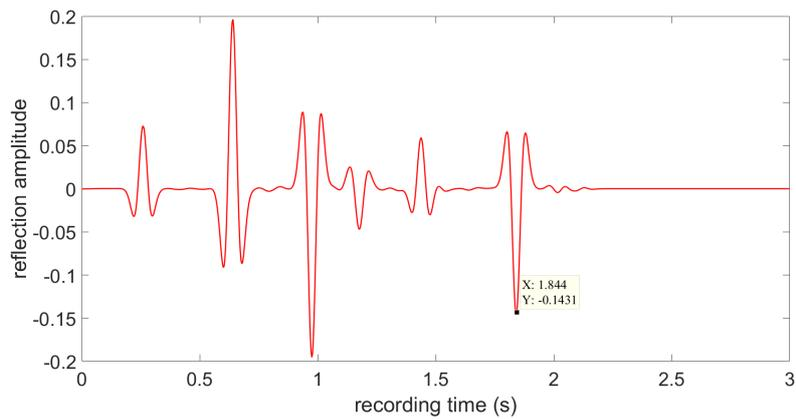
**Figure 6-5:** Upgoing focusing function exactly at the 7<sup>th</sup> layer at two-way travel time with the receiver at  $z_r = 280$  m
