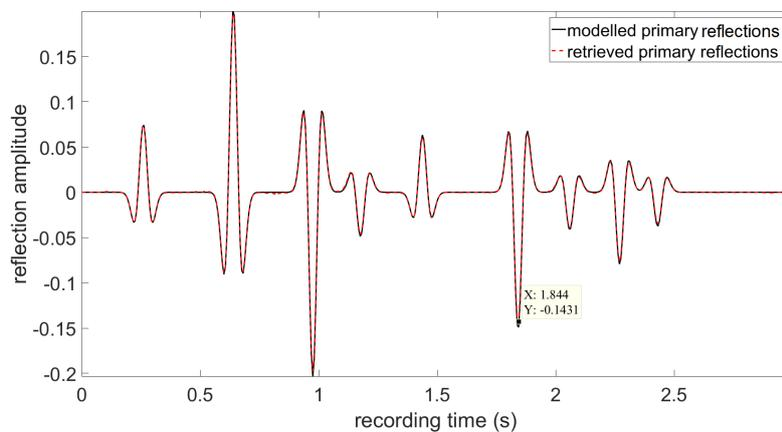
**Figure 6-6:** The obtained subsurface primaries (red dashed line) and the modelled reflectivity (black solid line) with the receiver at  $z_r = 280$  m convolved with the 20 Hz Ricker wavelet as a function of two-way travelttime
