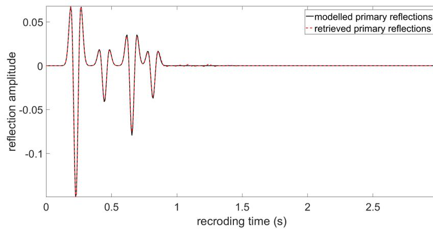
**Figure 6-14:** Modelled primaries (dark solid) and retrieved primaries (red dashed) at  $25^\circ$  incidence angle with source at  $z_s = 10$  m and receiver at  $z_r = 1700$  m
