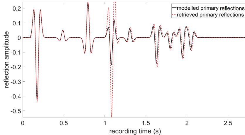
**Figure 6-12:** Modelled primaries (dark solid) and retrieved primaries (red dashed) at  $25^\circ$  incidence angle with source at  $z_s = 10$  m and receiver at  $z_r = 30$  m
