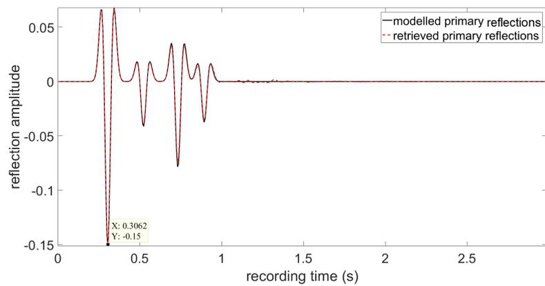
**Figure 6-10:** The obtained subsurface primaries (red dashed line) and the modelled reflectivity (black solid line) with the receiver at  $z_r = 1800$  m convolved with Ricker wavelet as a function of two-way traveltme
