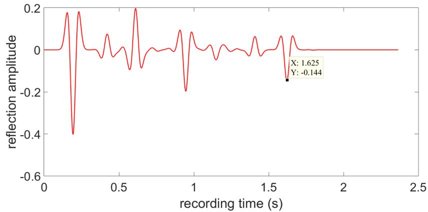
**Figure 6-1:** Upgoing focusing function exactly at the 7<sup>th</sup> layer at two-way travel time
