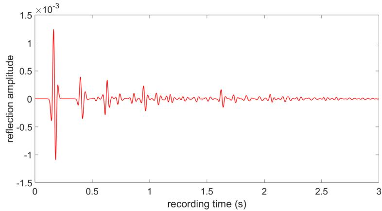
**Figure 6-4:** Modelled borehole vertical particle velocity convolved the 20 Hz wavelet with the receiver at  $z_r = 280$  m
