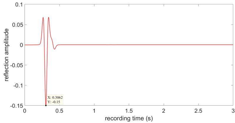
**Figure 6-9:** Projected focusing function exactly from the receiver to the 7<sup>th</sup> layer and back to the receiver with the receiver at  $z_r = 1800$  m
