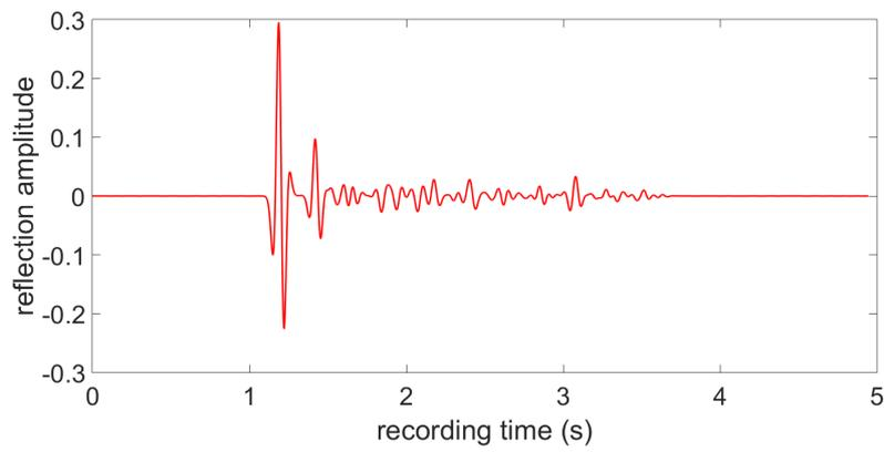
**Figure 4-6:** The obtained downgoing Green's function focusing at the 7<sup>th</sup> layer
