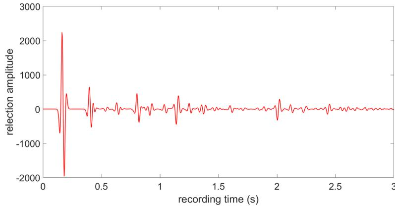
**Figure 6-3:** Modelled borehole acoustic pressure convolved with the 20 Hz wavelet with the receiver at  $z_r = 280$  m
