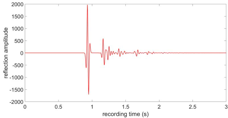
**Figure 6-7:** Modelled borehole acoustic pressure convolved with the 20 Hz wavelet with the receiver at  $z_r = 1800$  m
