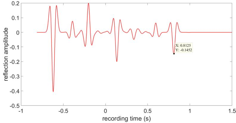
**Figure 4-3:** Upgoing focusing field at exactly the 7<sup>th</sup> layer
