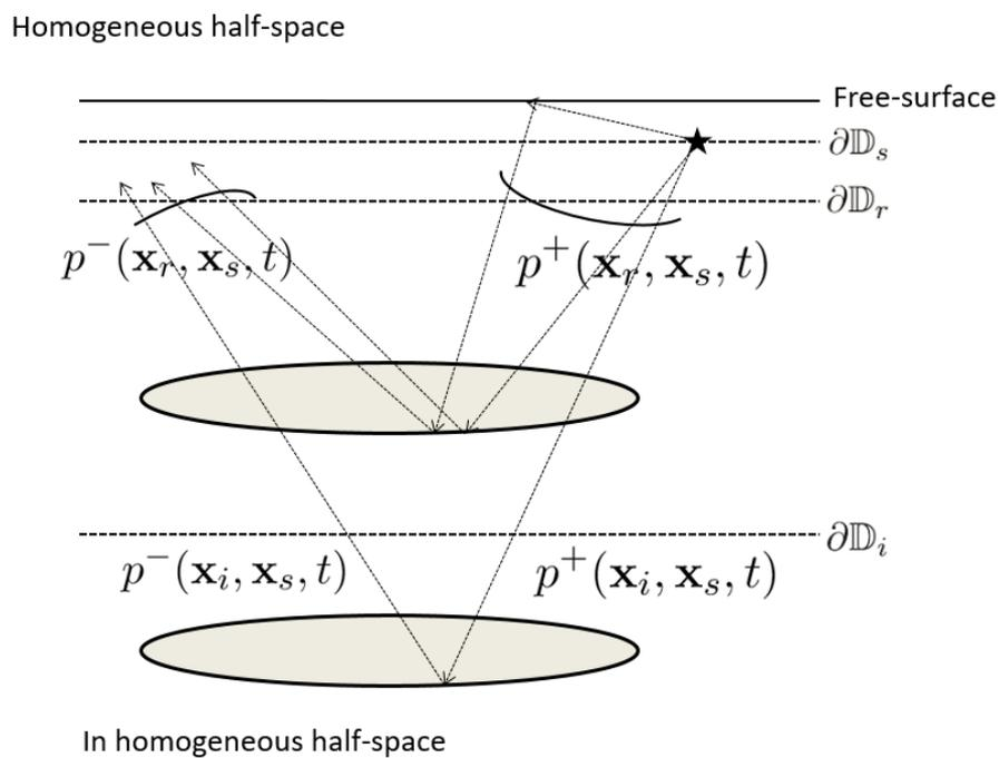
**Figure 2-6:** Downgoing and upgoing Green's functions in the actual medium including a free surface with different source and receiver depth levels
