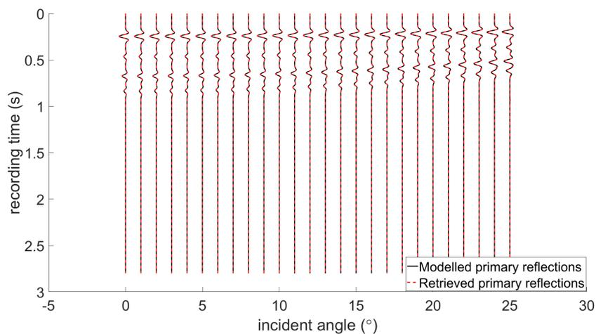
**Figure 6-13:** Gather of 'traces' with primaries as a function of two-way travel time with source at  $z_s = 10$  m and receiver at  $z_r = 1700$  m
