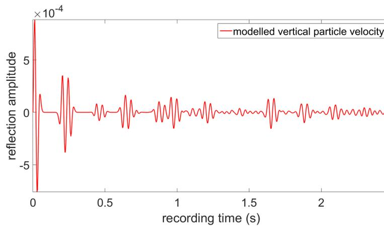
**Figure 4-2:** Modelled two-way vertical particle velocity convolved with the 20 Hz wavelet
