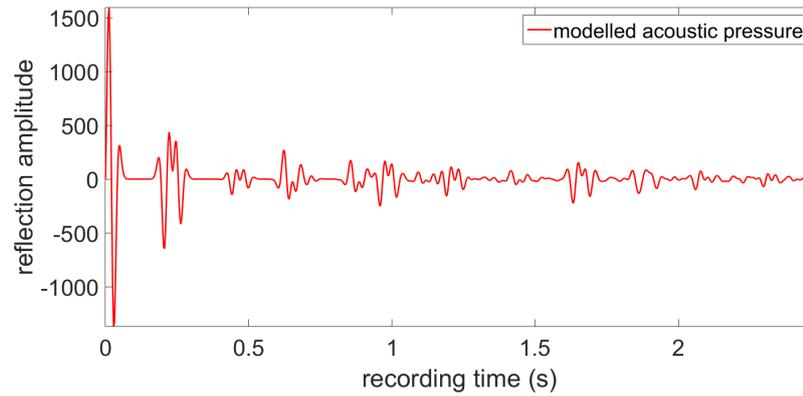
**Figure 4-1:** Modelled two-way acoustic pressure convolved with the 20 Hz wavelet
