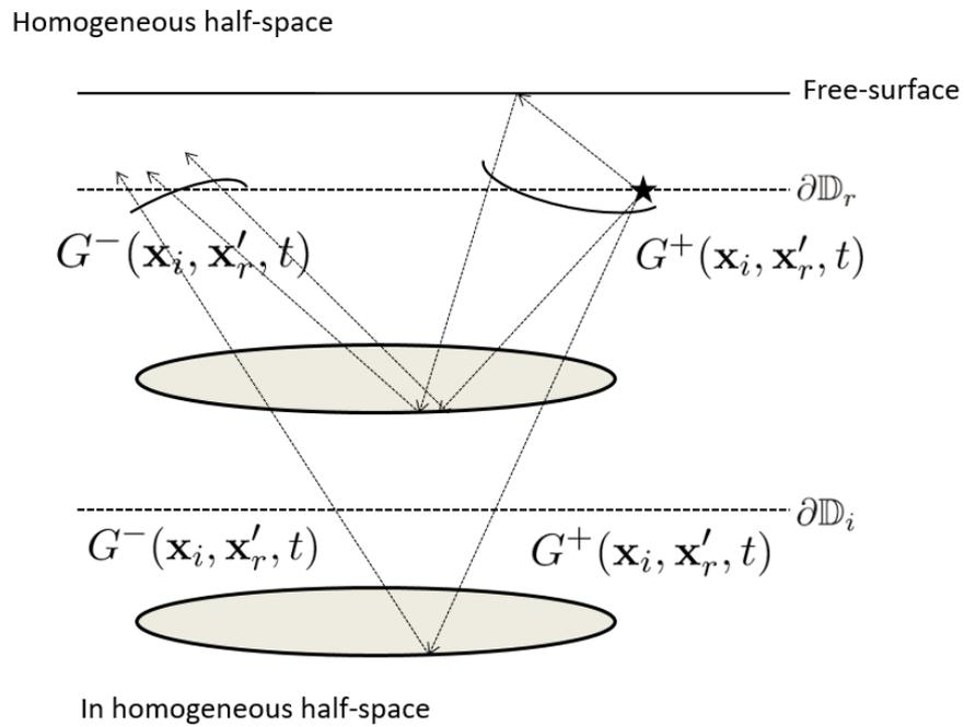
**Figure 2-5:** Downgoing and upgoing Green's functions in the actual medium including a free surface
