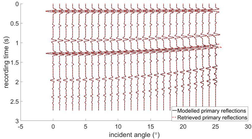
**Figure 6-11:** Gather of 'traces' with primaries as a function of two-way travel time with the source at  $z_s = 10$  m and the receiver at  $z_r = 30$  m
