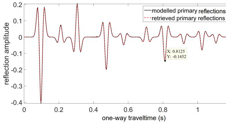
**Figure 4-4:** The obtained subsurface primaries (red dashed line) and the modelled reflectivity (black solid line) convolved with the 20 Hz Ricker wavelet as a function of one-way traveltme
