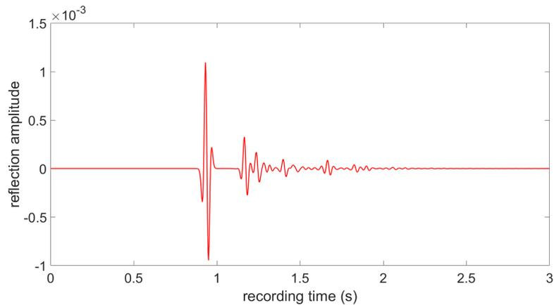
**Figure 6-8:** Modelled borehole vertical particle velocity convolved with the 20 Hz wavelet with the receiver at  $z_r = 1800$  m
