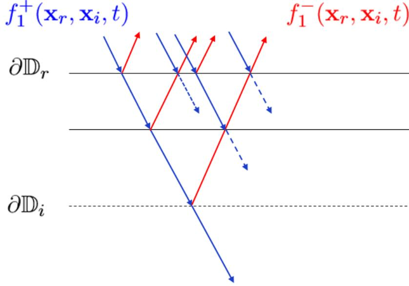
**Figure 2-4:** Illustration of up- (red) and downgoing (blue) focusing wavefields
