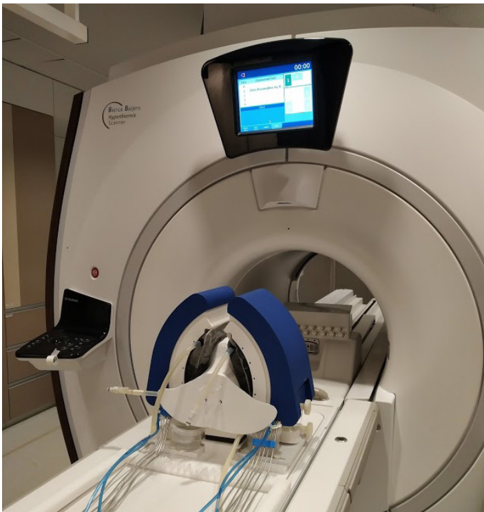
Fig. 81: MRcollar set-up in MR scanner
