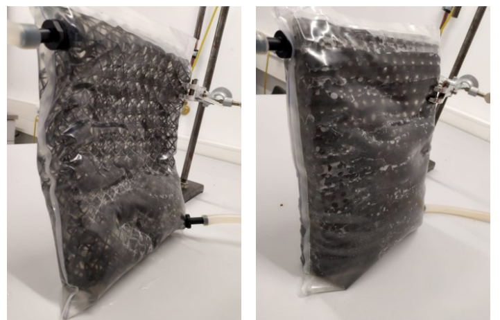
Fig. 74: Lattice vs. Honeygrid iteration 1 glue adhesion, while circulating with water
