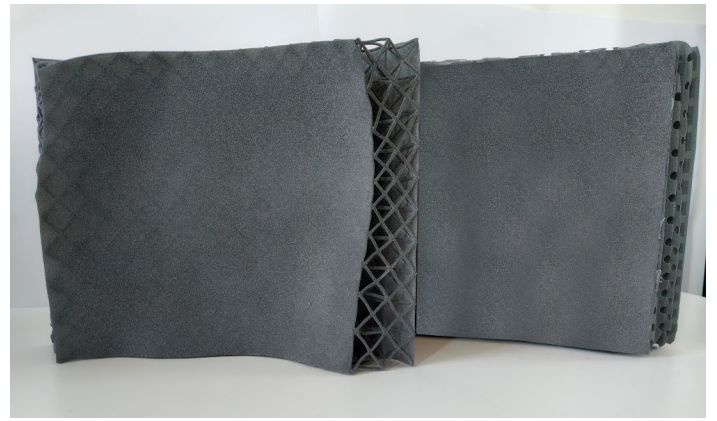
Fig. 75: Iteration 2: Fully closed glue surface
