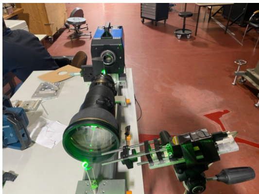
Fig. 22 Retro-reflective PIV setup with laser illumination (from the left) and the light trap behind the imaging lens (in the foreground on the right). A half aperture between camera and imaging lens serves as 'cutoff grid'.
