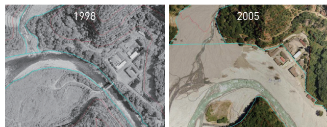
fig.18 Photos showing the damage caused by Typhoon in 2005, the power plant office and the dam was destroyed.
