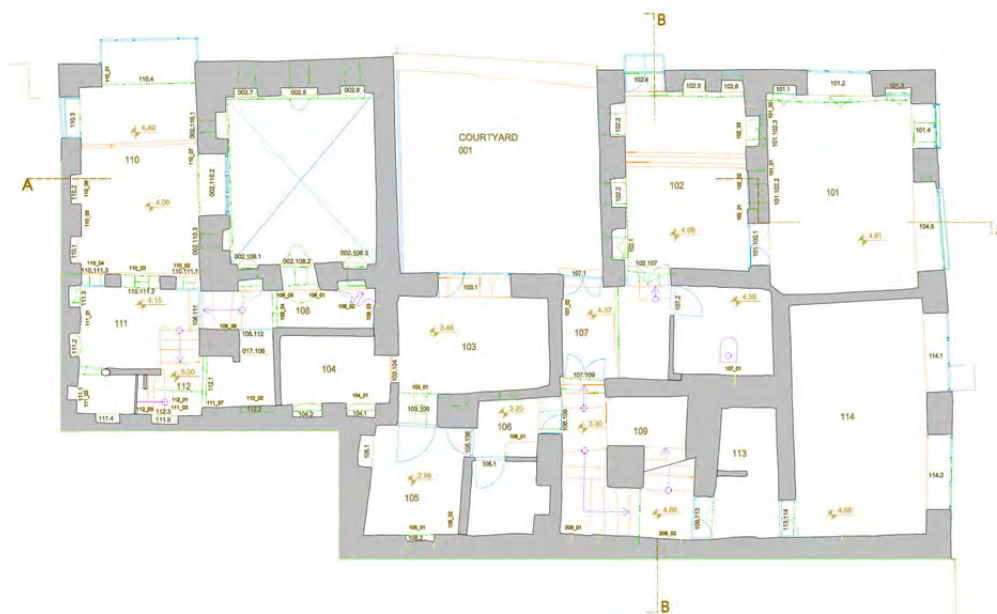
Figure 2: First floor of Al-Nawar House. The surveyed room 101 is located on the upper right corner in north-western direction. The façade openings are just filled with wooden shutters [3].
