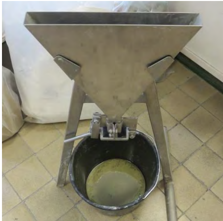
Figure 3: Determination of the V-funnel flow time of the mortars
