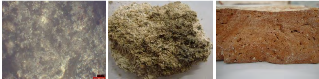
Capture 2: Salts in a sample of mortar (left), black crust (centre) and section of a brick (right).
