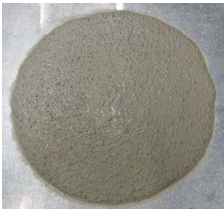
Figure 5: Unmodified reference (SCC) with appearance of separation
