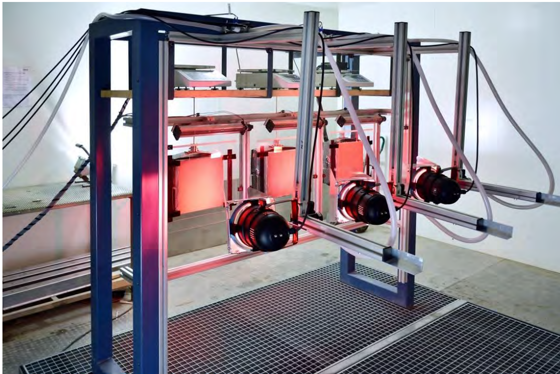
Figure 2: Custom-built machine for the reproduction of weathering conditions on a building facade
