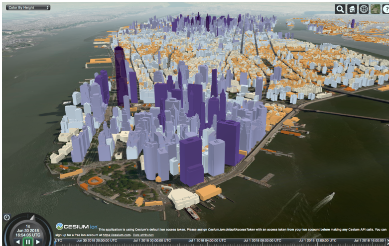
Figure 5.2: An application built on top of Cesium JS showing the buildings in New York city coloured according to their height value [Cesium, 2018].
