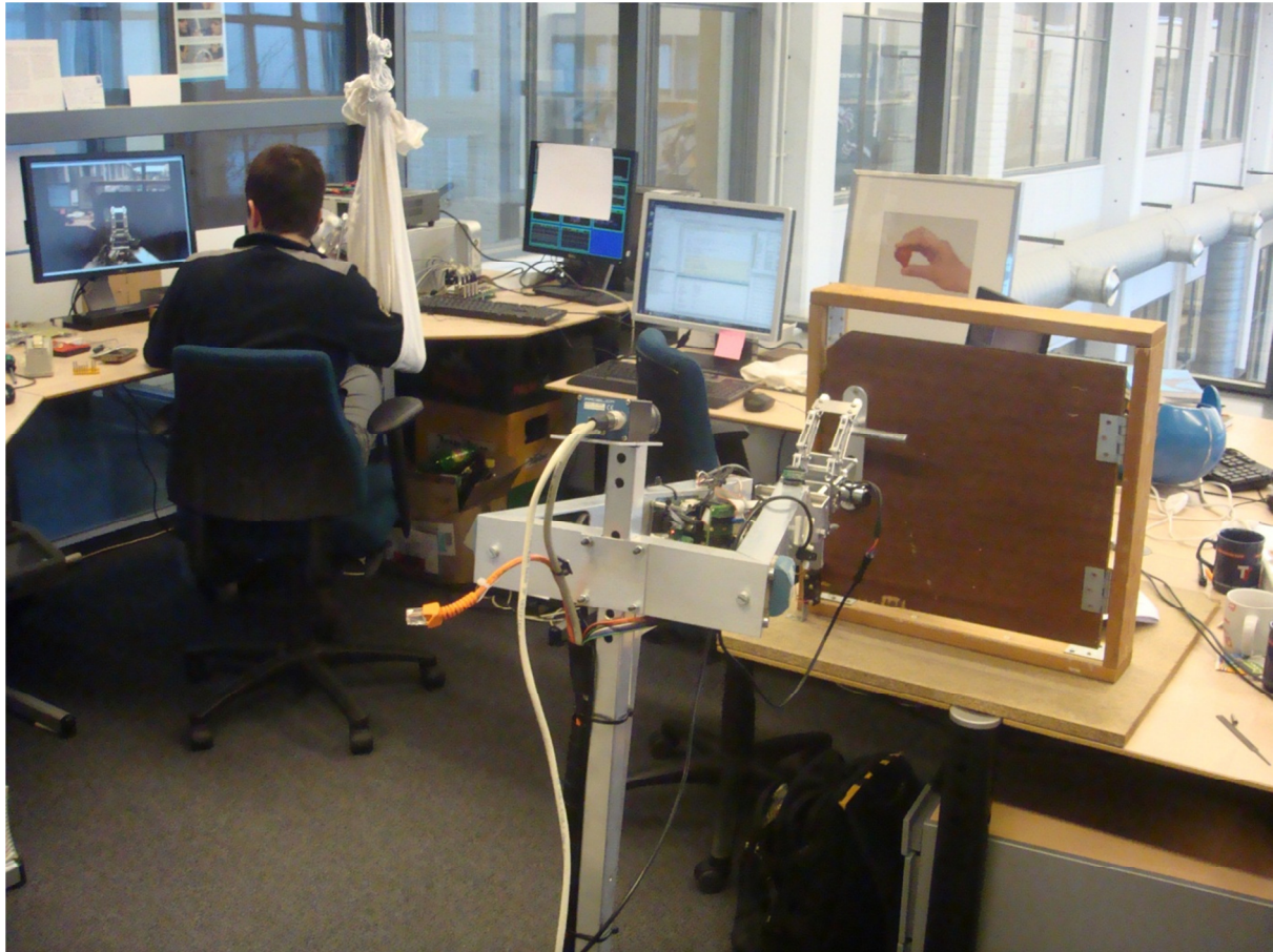
Figure A-28: An operator controlling the Delft Personal Robot 1 (DPR1) with the Delft Hand 3 (DH3) to open a table top door. DH3 has here less degrees of freedom and less compliance because two fingers have been locked together with a plate.
