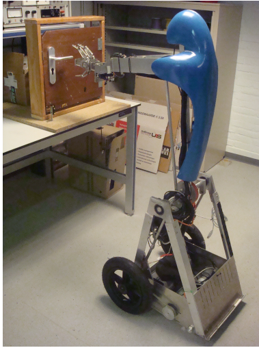
Figure 4 – Delft Personal Robot 1 (DPR1), the slave device used for the experiment, a 5 DOF non-holonomic, non-redundant service robot with an underactuated hand. In front of the robot is the table top door that was constructed for the experiment.
