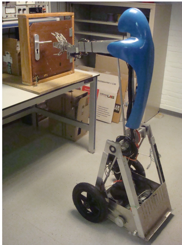
Figure A-3: Delft Personal Robot 1 (DPR1), the slave device used during the experiment of opening doors and the table top door created for the purpose of the experiment
