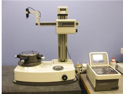
Figure 4.1.8 roundness measurement tool whose standard probe was replaced with a CCD camera and a lens system connected to a TV screen (not shown here) used to examine the concentricity between the optical elements.
