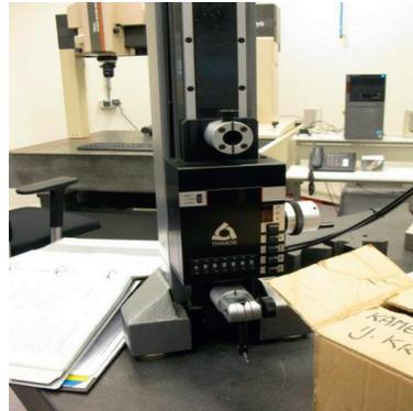
Figure 4.1.6a (left) 3D coordinate measurement tool and Figure 4.1.6b (right) height measurement tool.
