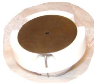
Figure 4.1.9 picture of the complete unit of electron source, E-1 and E-2 aligned and glued to the Macor.
