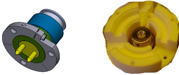
Figure 4.1.7a (left) mechanical drawing of the electron source fixed in its clamping ring and Figure 4.1.7b (right) a picture of the electron source mounted to the Macor (the electrical connection to the extractor is also clear from picture).
