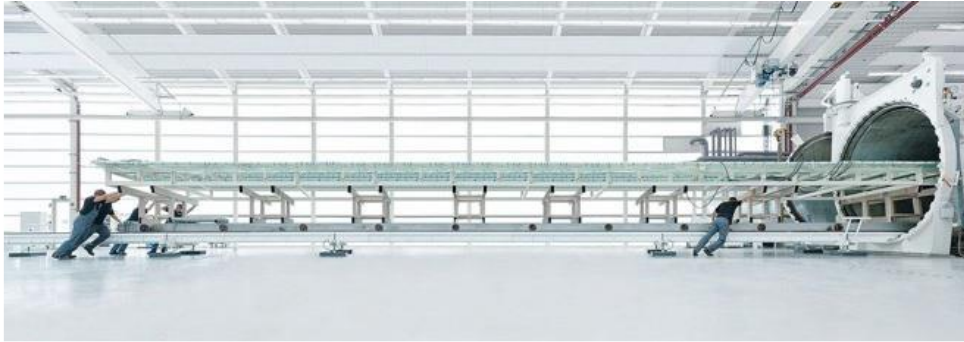
Figure 28: The largest glass industry autoclave (lamination up to 15m), Sedak Industry (Sedak, 2020)
