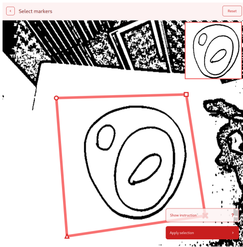
Figure 2: Isolating the level curves in the captured image, with the help of a preview in the top-right corner of the GUI.
